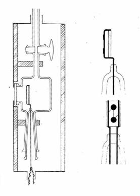
The vanes used in these thermocouples were made of thin aluminum foil, approximately 3.8 x 7 mm. in size. They were blackened with a coating of ordinary commercial dead-black lacquer. The junctions were made of fiwe bismuth-bismuth (10% tin) wires and were arranged six in series. Three junctions were attached to each vane by means of Du Pont "Household Cement". A piece of fluorescent uranium glass placed behind the vanes was a necessary aid in focussing the light.
