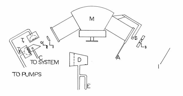
The analytical system was the same as that already described. It was joined thru a cut-off and a quartz pyrex graded seal to the cell C, the whole system being designed to keep the total volume as small as possible. The monochromator, cell and thermocouples were mounted on a table attached to the vacuum bench behind the analytical apparatus. The monochromator and spark set-up have already been described.
