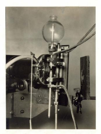
To prevent melting of the electrodes and overheating of the monochromator parts, a stream of compressed air was blown thru the spark in order to direct it away from the monochromator. The quantum yield experiments were carried out using the radiation of  $\lambda$  1990 exclusively, but the qualitative experiments for the detection of ammonia required the full radiation from an aluminum spark placed 20 cm. in front of the cell.
