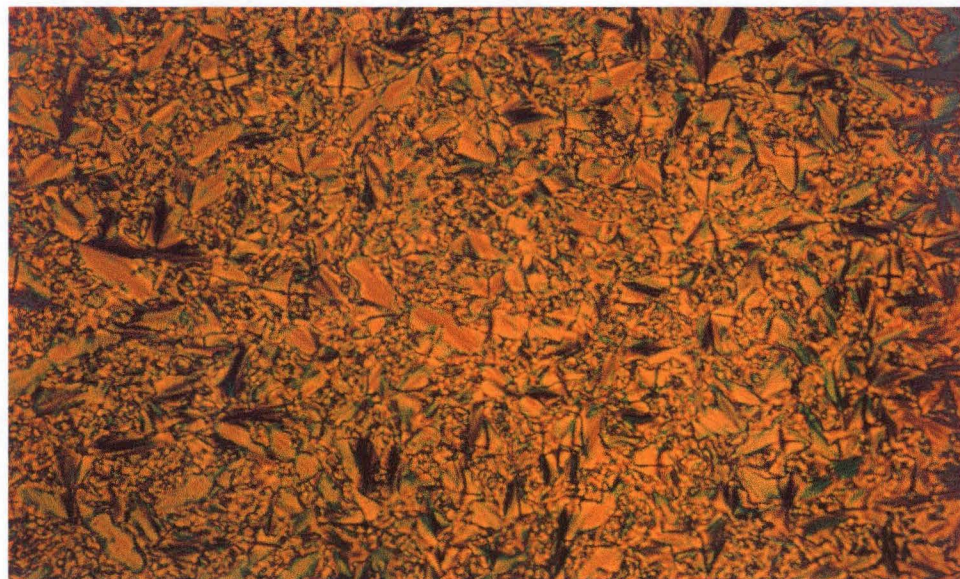
Figure 9b. Polarized optical micrograph (magnification 50x) of the regular smectic A texture observed on cooling 27 from the isotropic state at 110.3°C.
