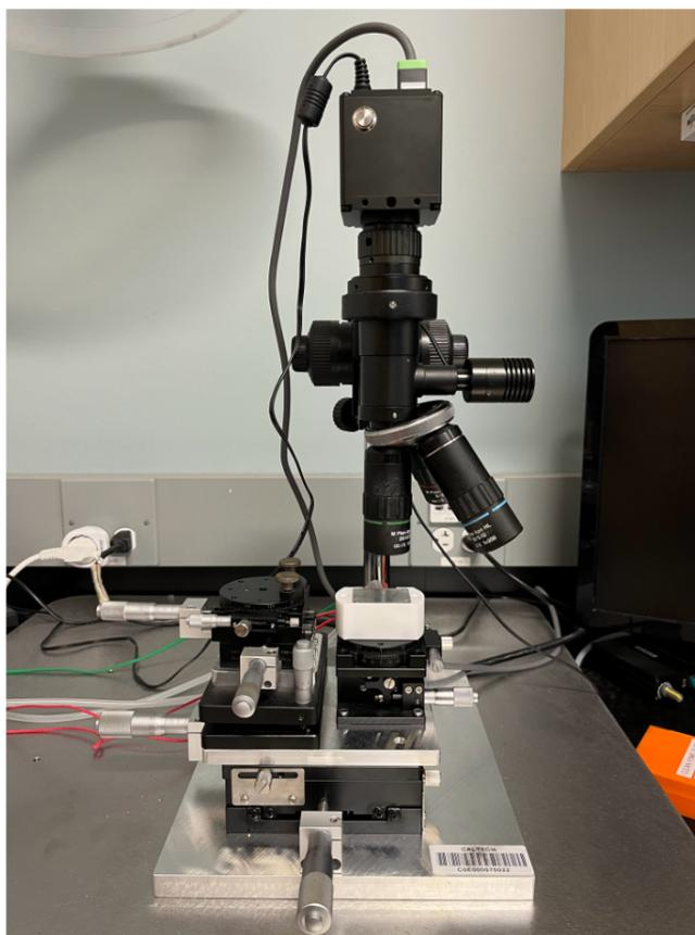
Figure 2.5: A transfer setup used to make van der Waals heterostructure stacks.
