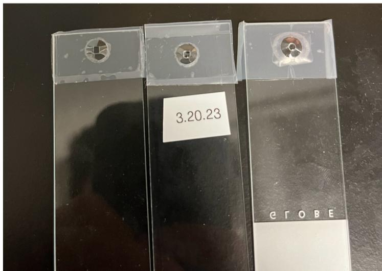
Figure 2.4: PC/PDMS stamps. Optical images of PC/PDMS stamps. From left to right are PC on flat PDMS stamp, PC on domed PDMS stamp, and also polypropylene carbonate (PPC) on domed PDMS stamp.
