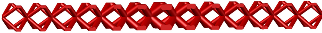
Figure 1.3: Example of a functionally graded lattice material. The gradients are created by changing the lattice parameters. Adopted from [3].
