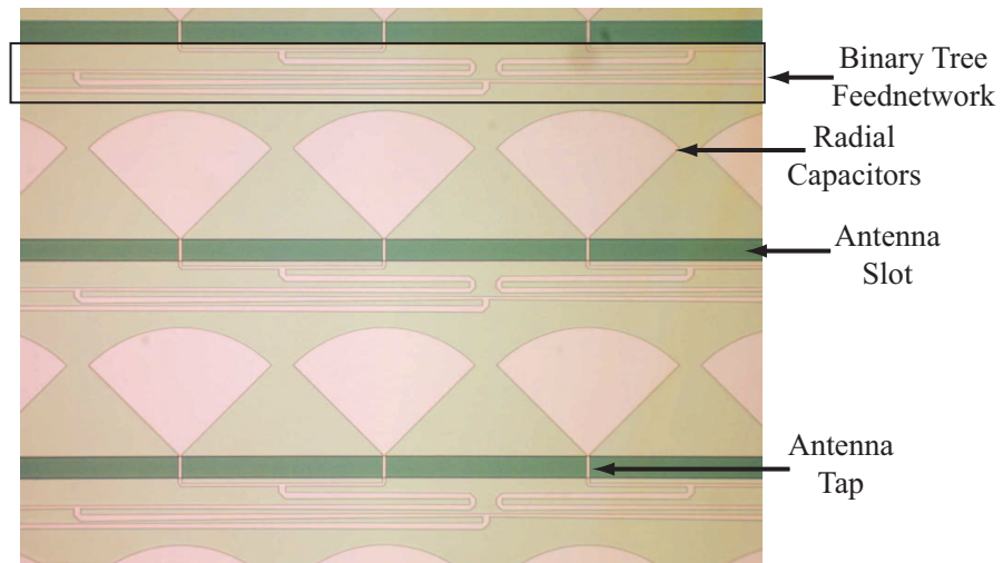
Figure 3.8: Optical image of the antenna slot and the feednetwork taken under the microscope
