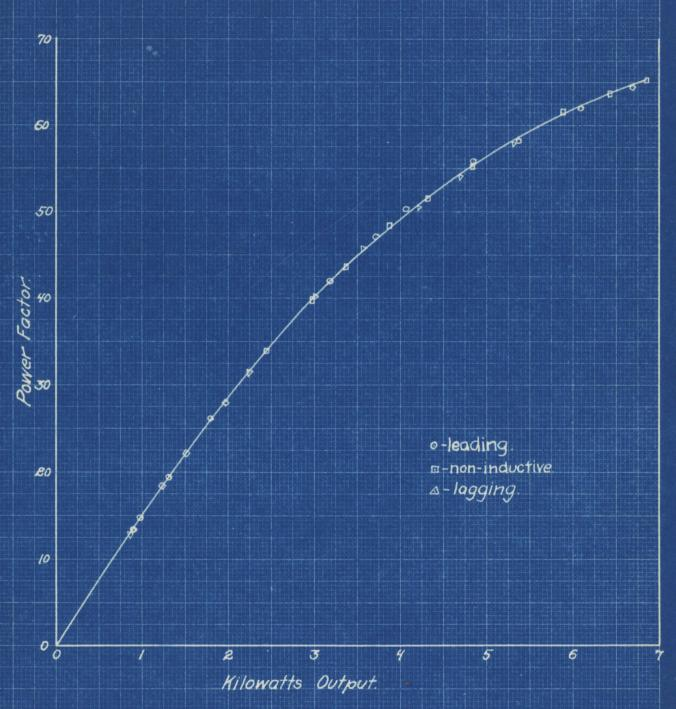
Quadrature and Exciting Current Curves Induction Generator loaded with leading lagging and non-inductive loads. Synchronous motor supplying quadrature current. 110 volts- 50 cycles.
