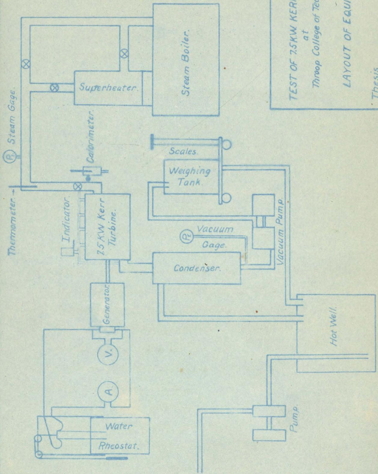
TEST OF 75KW KERR TURBINE.
