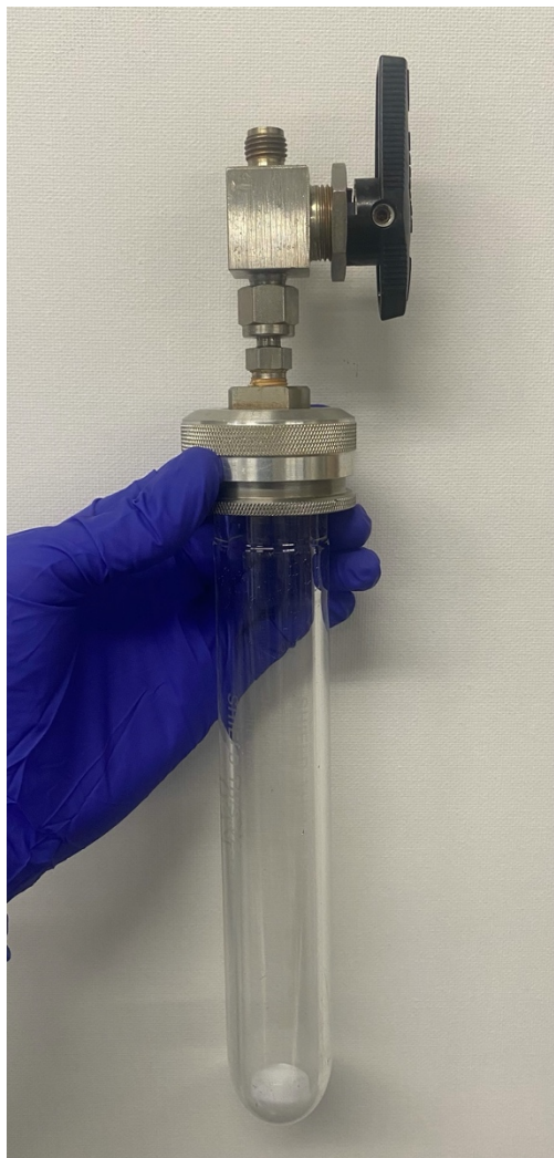
Figure D2: Photograph of a custom-built high pressure reaction vessel used for photolytic reactions.
