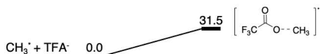
Figure E7: DFT free energy barrier for the methyl radical to combine with a free TFA anion to generate a MeTFA radical anion.
