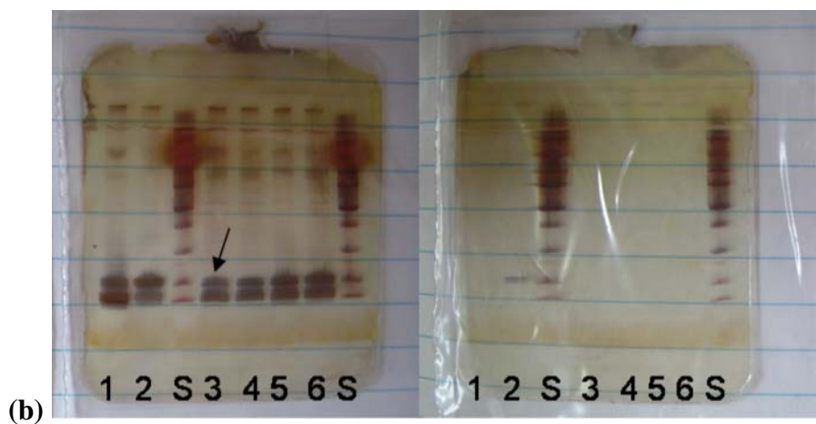
Figure 7.9. SDS-PAGE of WT only (lane #1), A30P only (lane #2), standard (lane #S), WT + Y19/W39 (lane #3), WT + Y19(NO 2 )/W39 (lane #4 and #5), and A30P + Y19/W39 (lane #6) at (a) Day 6 and (b) Day 9 from reaction mixture (left) and supernatant (right). Monomeric species are indicated by arrows.
