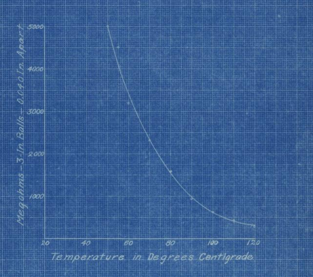
Effect of Temperature on the Dielectric Strength of Transformer Oil
