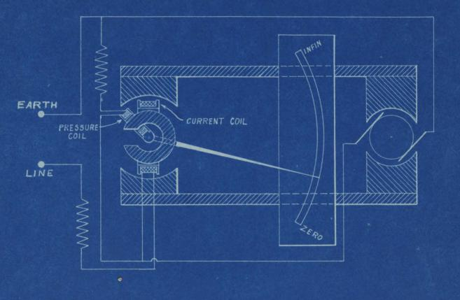
Arrangement of Apparatus
