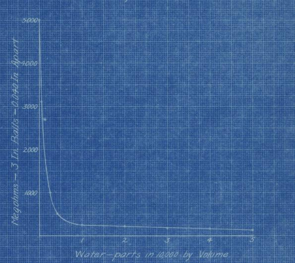
Relation between Megger Reading and Dielectric Value of Transformer Oll as Moisture is Added. Temperature = 55°C.
