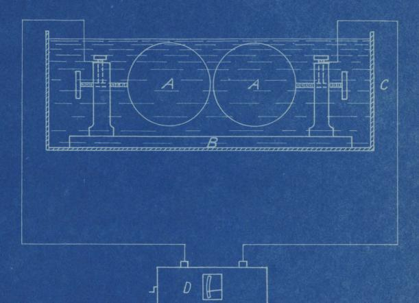
AA-3" Hollow copper spheres B-Base of sphere gap—composition board C-Container for gap and oil D-Megger
