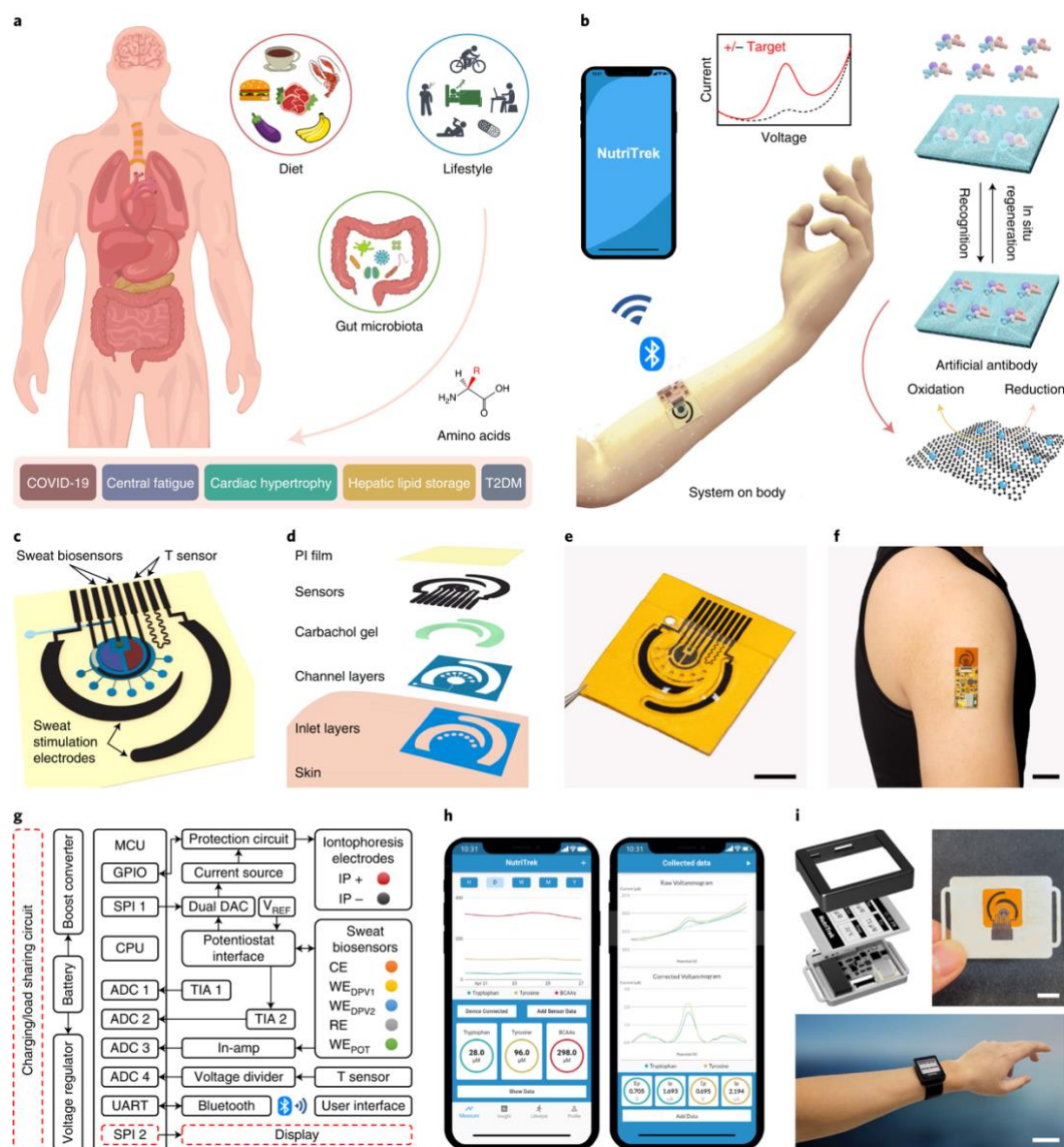
Figure 5-1: a , Circulating nutrients such as AAs are associated with various physiological and metabolic conditions. b , Schematic of the wearable ‘NutriTrek’ that enables metabolic monitoring through a synergistic fusion of LEG, RARs and artificial antibodies. c,d , Schematic ( c ) and layer assembly ( d ) of the microfluidic ‘NutriTrek’ patch for sweat induction, sampling and biosensing. T, temperature. e,f , Images of a flexible sensor patch ( e ) and a skin-interfaced wearable system ( f ). Scale bars, 5 mm ( e ) and 2 cm ( f ). g , Block diagram of electronic system of ‘NutriTrek’. The modules outlined in red dashes are included in the smartwatch version. CPU, central processing unit; POT, potentiometry; In-Amp, instrumentation amplifier; MCU, microcontroller; TIA, trans-impedance amplifier; IP, iontophoresis; CE, counter-electrode; RE, reference electrode; WE, working electrode. h , Custom mobile application for real-time metabolic and nutritional tracking. i , ‘NutriTrek’ smartwatch with a disposable sensor patch and an electrophoretic display. Scale bars, 1 cm (top) and 5 cm (bottom).
