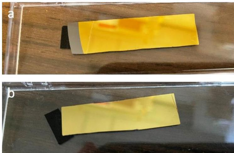
Figure 7.12. Laminate nanoparticle films of (a)  $\text{SiO}_2$  and (b)  $\text{Si}_3\text{N}_4$  deposited by nonthermal plasma synthesis onto gold coated substrates. The samples are approximately 1 cm wide and 4 cm long.
