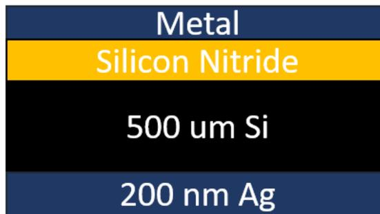
Figure 2.10. Schematic of a metal AR coated selective solar absorber.
