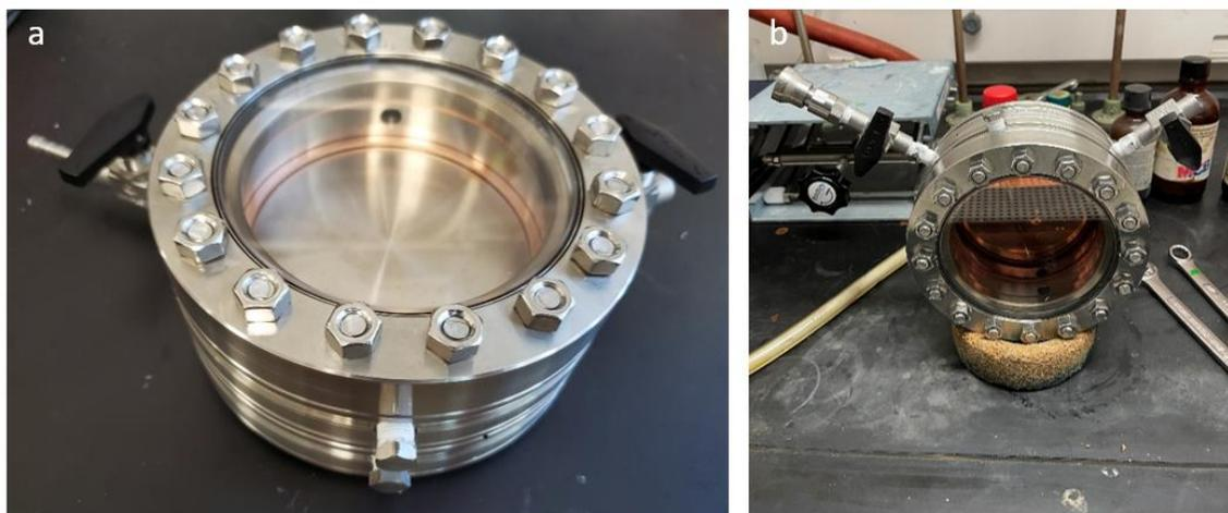
Figure 3.11. Fully constructed photothermal reactor in batch mode setup. Two quarter-turn valves with Quick Connect valves are attached. The other ports are sealed with plugs. Note that the selective solar absorber is not installed in (b).
