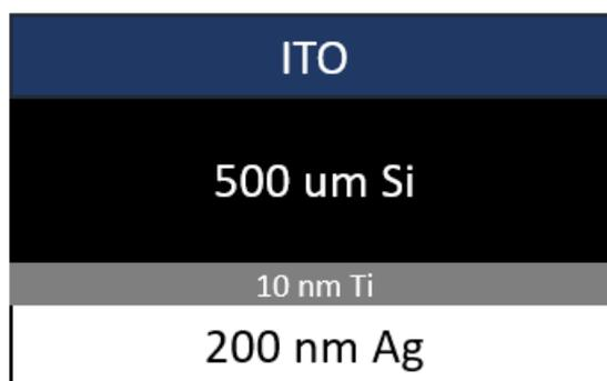
Figure 2.6. Schematic of an ITO-based selective solar absorber.
