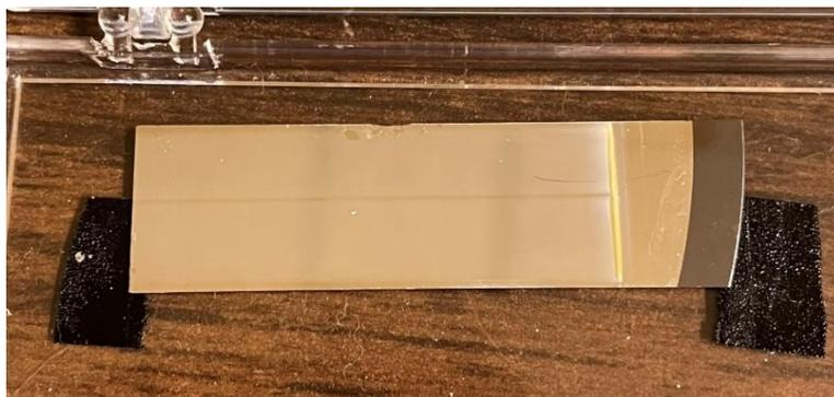
Figure 7.18. Image of  $\text{Si}_3\text{N}_4$  laminate nanoparticle film on silver substrate deposited from nonthermal plasma synthesis with 400 raster passes. The sample size is approximately 1 cm by 4 cm.
