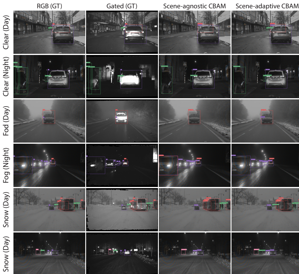
Figure 8.5: Object detection results on STF dataset in various scene conditions. From top to bottom: RGB images, gated images, scene-agnostic CBAM detections, and scene-adaptive CBAM detections. RGB and gated images are overlaid with ground truth bounding boxes.
