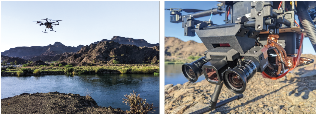
Figure 4.4: Our UAV operating over the Colorado River, CA, and the sensor stack mounted to the UAV showing the time-synchronized FLIR ADK thermal camera and VN100 IMU. Visible light cameras were not used as part of this work.
