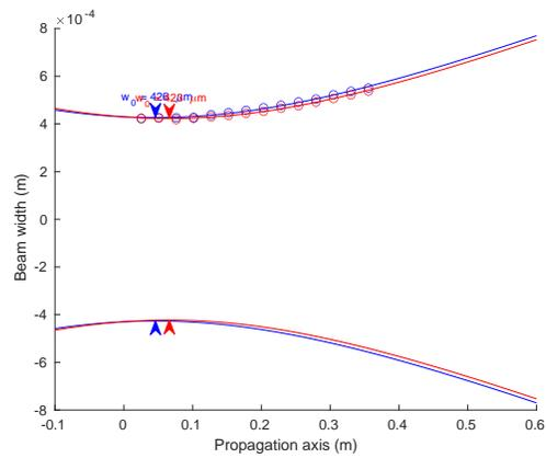
Figure 8.7: Beam profile of probe laser showing good agreement (ellipticity close to 1) along two transverse axes.
