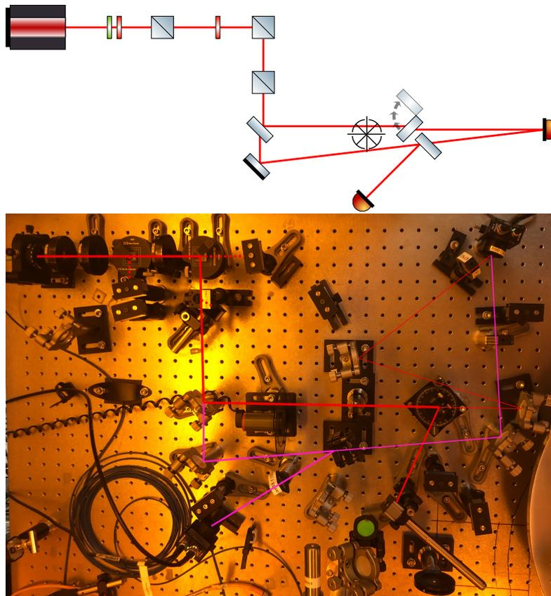
Figure 8.4: Optical layout for mirror transmissivity measurement
