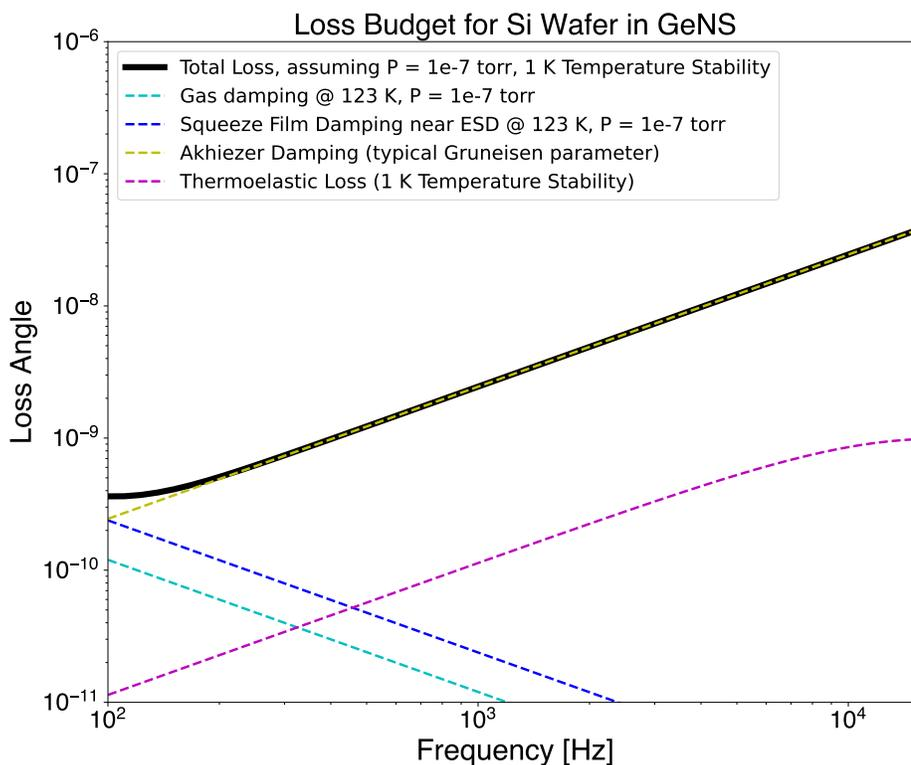
Figure 7.5: Mechanical loss budget for a bare Si wafer with 2" diameter, held at  $123 \pm 1$  K and mechanically isolated from the environment with a gentle nodal suspension.
