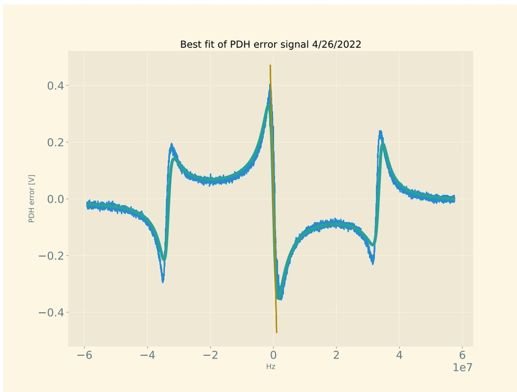
Figure 9.1: PDH error signal fitted to find a frequency discriminant of 2.2 MHz/V.
