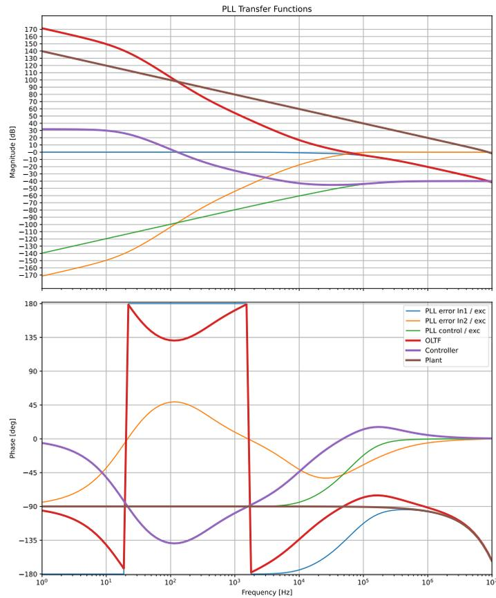
Figure 9.9: Bode plots of the phase-locked loop stabilizing pump-probe beat frequency on REFL photodiode. Excitation is summed at the PLL error point, with In1 just before and In2 just after the summation point. OLTF, Controller, and Plant are open loop transfer function.
