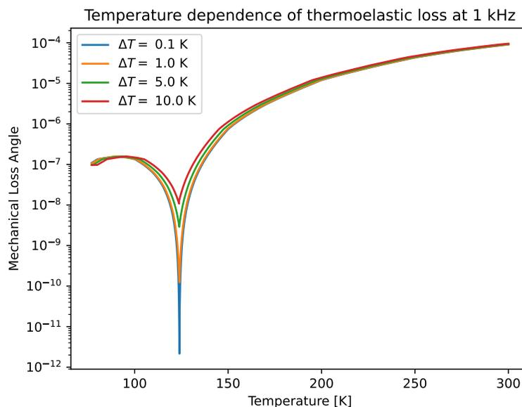
Figure 7.1: Mechanical loss at 1 kHz for a 2” silicon wafer due to thermoelastic damping, limited to the worst mechanical loss within  $\Delta T$  K of the nominal system temperature. One can see that near 123 K where thermoelastic loss sharply decreases, temperature stability can limit the lowest achievable thermoelastic loss. However,  $\pm 1$  K is not a terribly stringent requirement.
