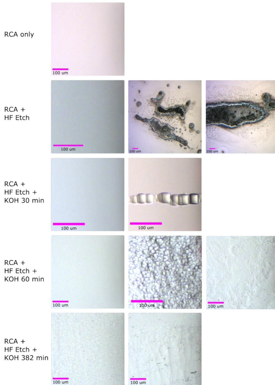
Figure 5.2: The stills captured from the AFM's video microscope are ordered from top to bottom by increasing KOH etch time, starting with RCA-cleaned samples with no HF or KOH etching. The left-most column are taken near the location of the AFM scan quoted in the roughness measurements. The other columns show pitting or contamination elsewhere on the sample.
