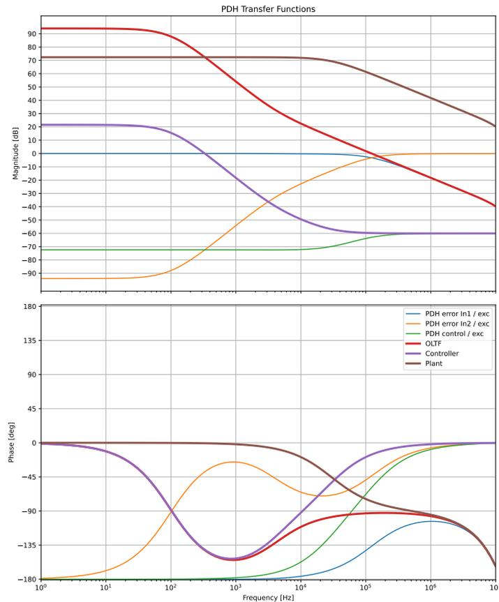
Figure 9.8: Bode plots of PDH loop in Finesse3 model. Excitation is summed at the PDH error point, with In1 just before and In2 just after the summation point. OLTF, Controller, and Plant are the open loop transfer functions.
