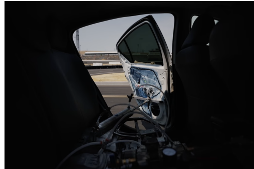
(d) Instrumented door to test whether Zoox car can properly detect and avoid collision.
