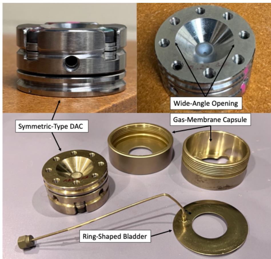
Figure 2.4: (Upper Left) Front view of the symmetric-type diamond-anvil cell (DAC). (Upper Right) Bottom view of the symmetric-type DAC displaying wide-angle opening. (Lower) Gas-membrane system used to make remote pressure changes.
