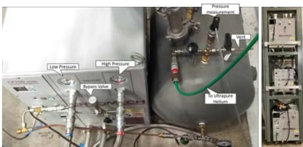
Figure 4.39: Photographs of the Cryomech Compressor System. Left, the CP103 compressor with the Buffer tank. Right, the three compressors in their tower.
