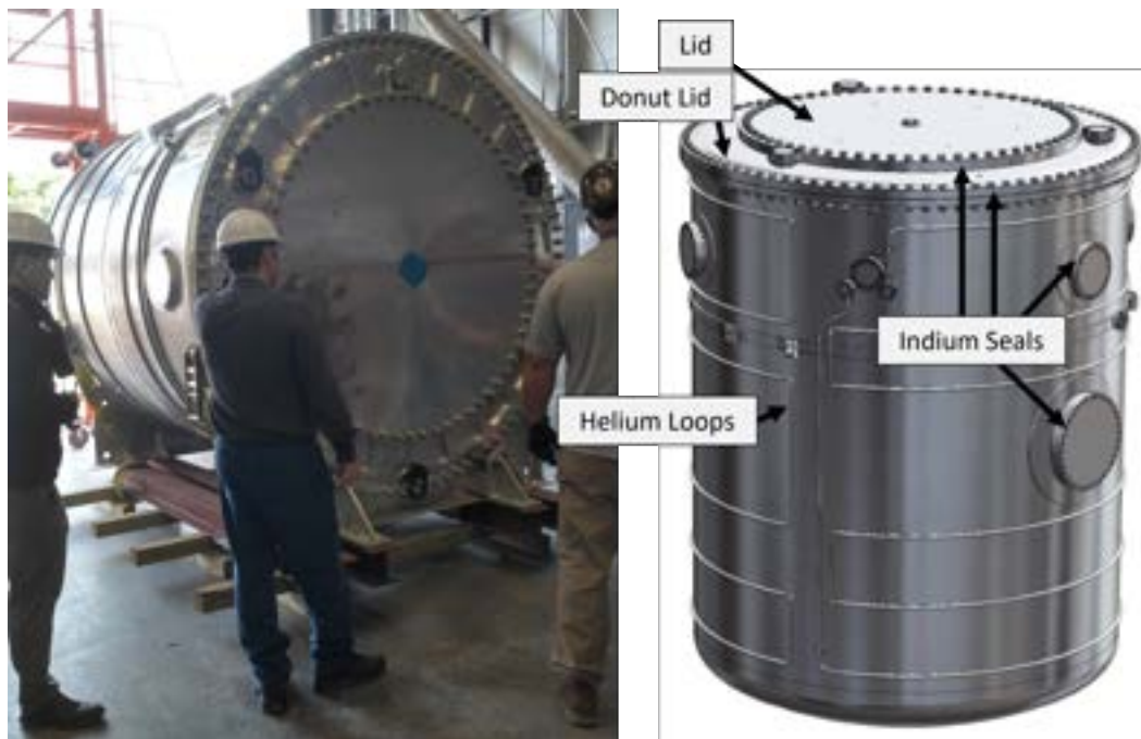
Figure 4.28: Inner Magnet Volume: Left, photograph of the IMV as shipped (on its side). Right, model of the IMV with its double lid, beam ports, and helium loops labeled.
