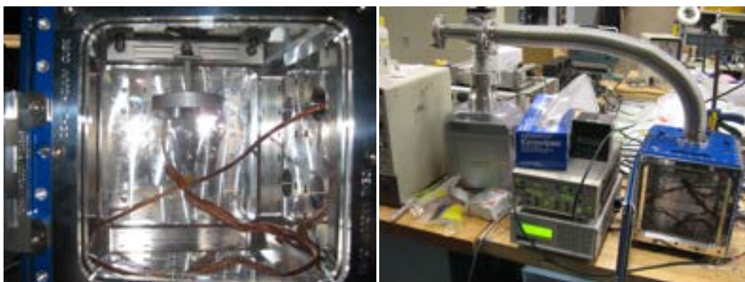
(a) Inside the Vacuum Test Box
