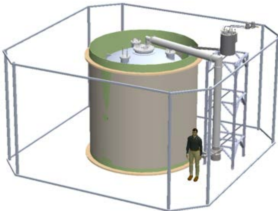
Figure 4.46: Computer Aided Design of the Magnet System. Note the large pipe (“trunk”) going from the top of the OVC to the manifold on the side.
