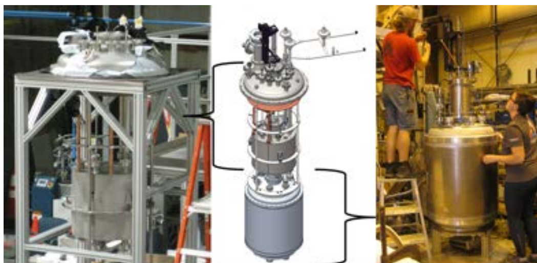
Figure 3.26: Center: CAD model of the Cryogenic Insert for the Cavallo Cryogenic Test Apparatus. Left: Photograph of the refrigerator for the insert at present. Right: Photograph of the CV for the insert being used at room temperature, with hard working students for scale.
