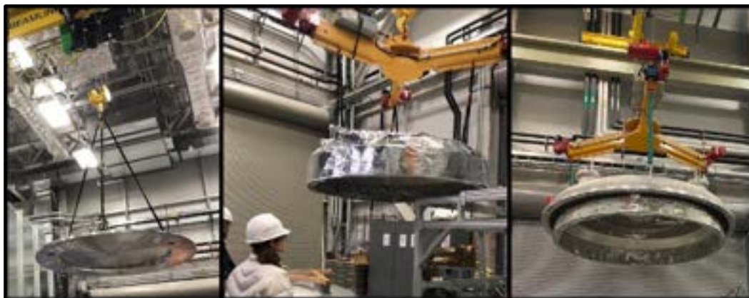
Figure 4.32: Lid installations. Left, the IMV lid before the magnetic field probe array is installed. Middle, the nitrogen shield mushroom (lid) covered in MLI, being craned by graduate student Marie Blatnik. Right, the OVC lid with the nitrogen shield mushroom attached.
