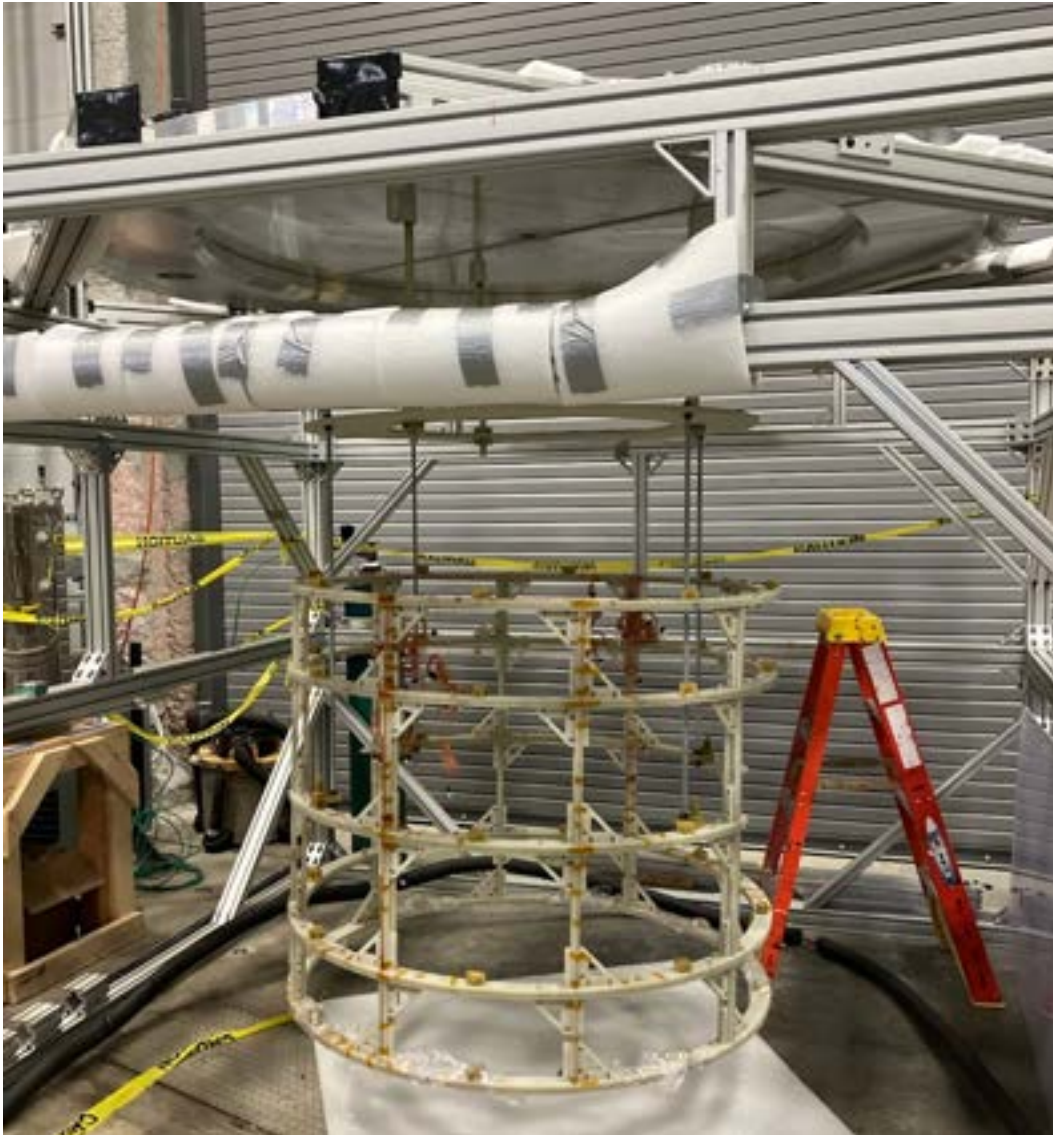
Figure 4.33: Photograph of the magnetic field probe array hanging from the IMV lid.
