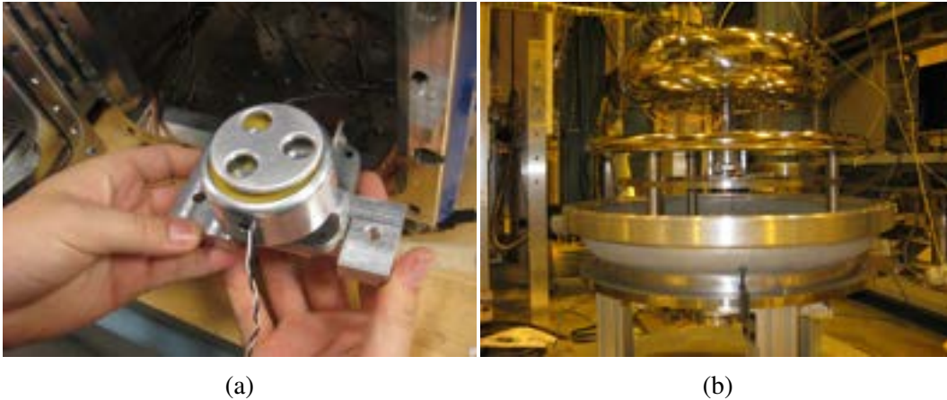
Figure 3.50: Robust Field Mill for the Cryogenic Cavallo Apparatus. Left: Photograph of the cryogenic field mill before installation. Right: The field mill was installed underneath the center hole in the D electrode.
