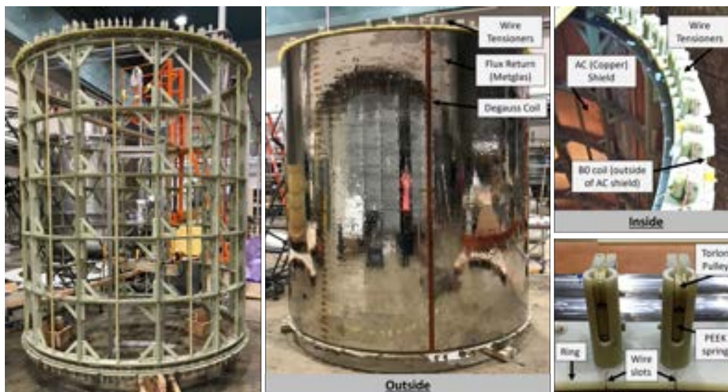
Figure 4.3: The Magnet Package, with emphasis on B0. Left, the B0 coil wound in its G10 support frame. Center, the outside of the magnet package, with the wound Metglas outer layer. Top right, the inside view of the magnet package, with the (currently innermost) AC shield layer. Bottom right, a close-up view of the wire tensioners made of Torlon pulleys and PEEK springs.
