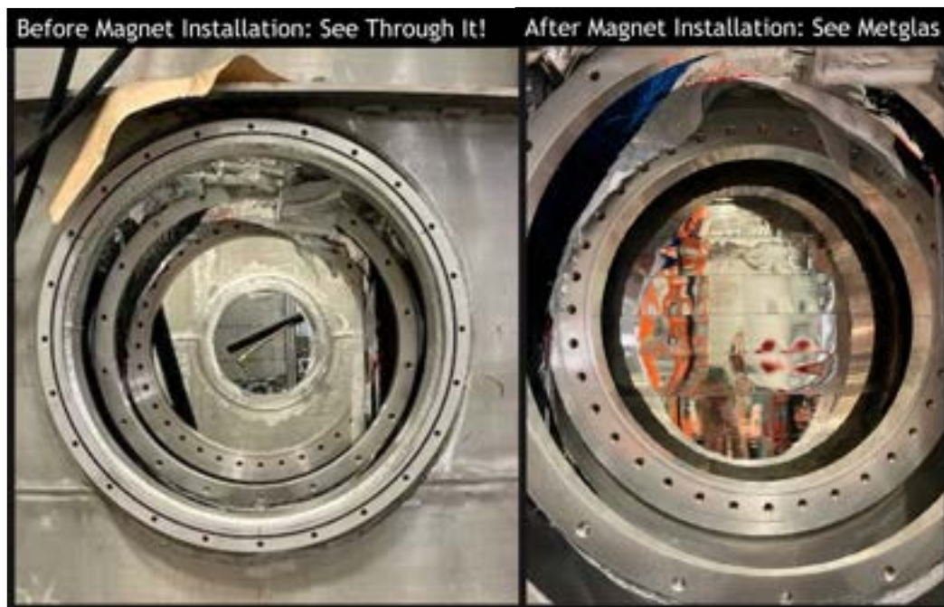
Figure 4.31: View through the open beamports before (left) and after (right) the magnet package was installed in the cryostat. The beam window flanges are not installed, allowing a view straight through the apparatus without the magnet package. Note, however, with the magnet package installed, the view is blocked by the Metglas flux return.
