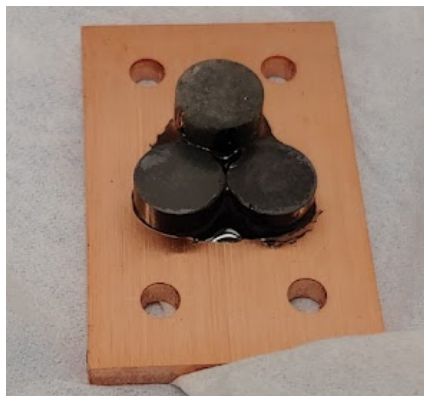
Figure 3.5: Example of a target plate with three fresh targets. These are targets with different ratios of \text{Yb}(\text{OH})_3 and Yb Powders, glued on with Stycast. The black color of the target mostly came from the Yb Powder.
