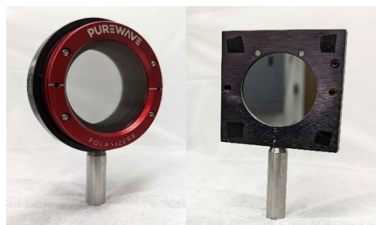
Figure 2.11. Wire grid polarizer with 12.5\ \mu\text{m} spacing (left) and mounted high resistivity (>10 kOhm) silicon wafer (right).
