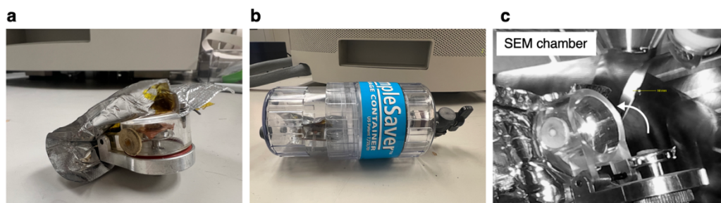
Figure 3.13 Optical images of a) Vacushut, a tool for air-free sample transfer from glovebox to SEM chamber, and b) Vacushut sealed in a secondary container. c) Vacushut lid opens in SEM chamber.
