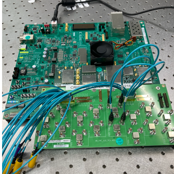
Figure B.3: A photograph of the QICK System based on Xilinx's ZCU216.
