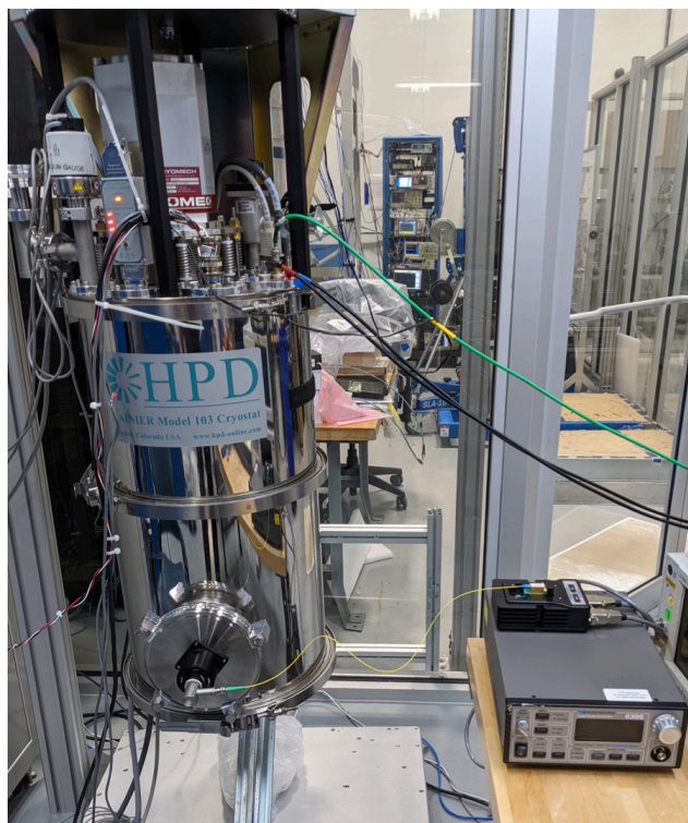
Figure 9.20: A picture of the laser diode controller, fiber-based laser diode, and reflective collimator attached on the ADR is shown.
