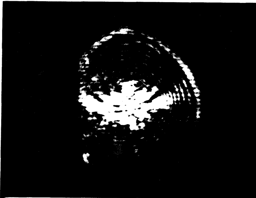
(d) Beam obtained when PPCM is replaced by an ordinary mirror.
