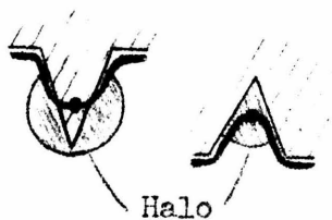
Fig. 1.10 BEAM CUTTING SHARP CORNERS
