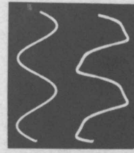
(a) TOP: NEAR SINEWAVE BOTTOM: TOO MUCH NEGATIVE RESISTANCE
