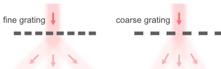
Figure 1.3: Light diffraction when interacting with a grating.
