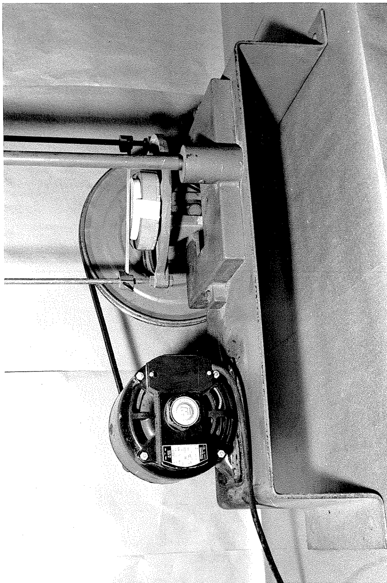
Figure 51 : Set-up used to smooth out the angularities of the carbon grains grade B - B - 6.
