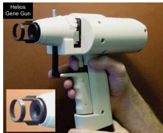
Figure 1.3: Schematic for the Bio-Rad Helios gene gun. Standoff distance shown is 2.8 cm. Reprinted with permission from O'Brien. 15
