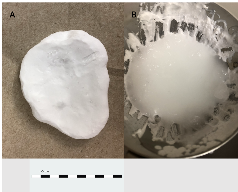
Figure 2.7: Brines frozen at liquid nitrogen temperatures in an inert nitrogen environment. A. MgCl 2 brine flash frozen via submersion in liquid nitrogen. The outer layer has a lower water concentration with the interior existing as a viscous fluid. B. MgCl 2 frozen by squeeze bottle spray into a liquid nitrogen cooled mortar. Flash freezing via this method causes ice build-up on the walls as well as slurry formation.
