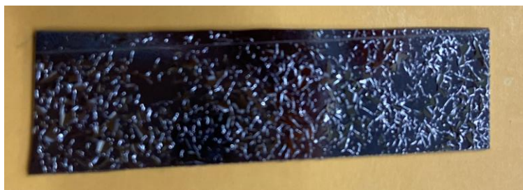
Figure A1. Example of silicon nanoparticles deposited on an Ag substrate and annealed at 800C for 1 hour.
