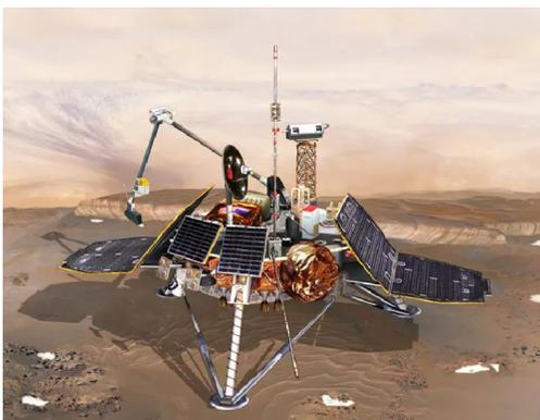
(d) Mars Polar Lander: vibrations during descent triggered touchdown sensor, causing premature landing thruster shutdown and loss of lander [6].
