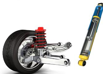
(g) Viscous Damper: dissipates energy through resistance of viscous fluid. Ex: car suspensions.
