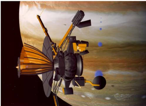
(c) Galileo Orbiter: lubricants worn away during transport vibration resulted in antenna deployment failure [5].
