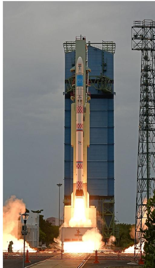
(e) ISRO Small Satellite Launch Vehicle D1: vibrations during stage separation triggered safe mode, preventing rocket from reaching intended orbit [7].
