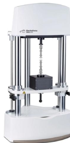
(b) Electroforce 3200 Dynamic Mechanical Analysis (DMA) Tester.
