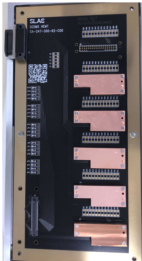
Figure 2.22: A photo of the HEMT-testing motherboard mounted in the bottom of its aluminum case. Five copper covers can be seen with HEMT mezzanine boards underneath. The two cable connectors can be seen on the top and bottom left.
