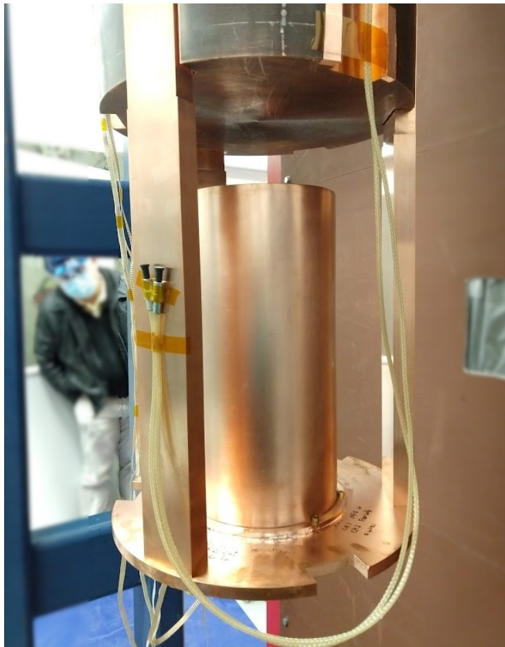
Figure 3.14: A photo of the copper enclosure holding the Run 3 detectors. The bottom copper plate is the same bottom plate from Figure 3.13. The Inner lead shield can be seen above the cylindrical copper housing. Three vertical bars thermally connect the bottom plate the the mixing-chamber stage of the dilution refrigerator (above the inner lead shield).
