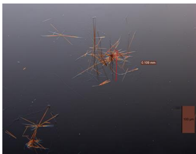
Figure H.14. Microscope image of the crystals used to attain the MicroED structure for 2-di .
