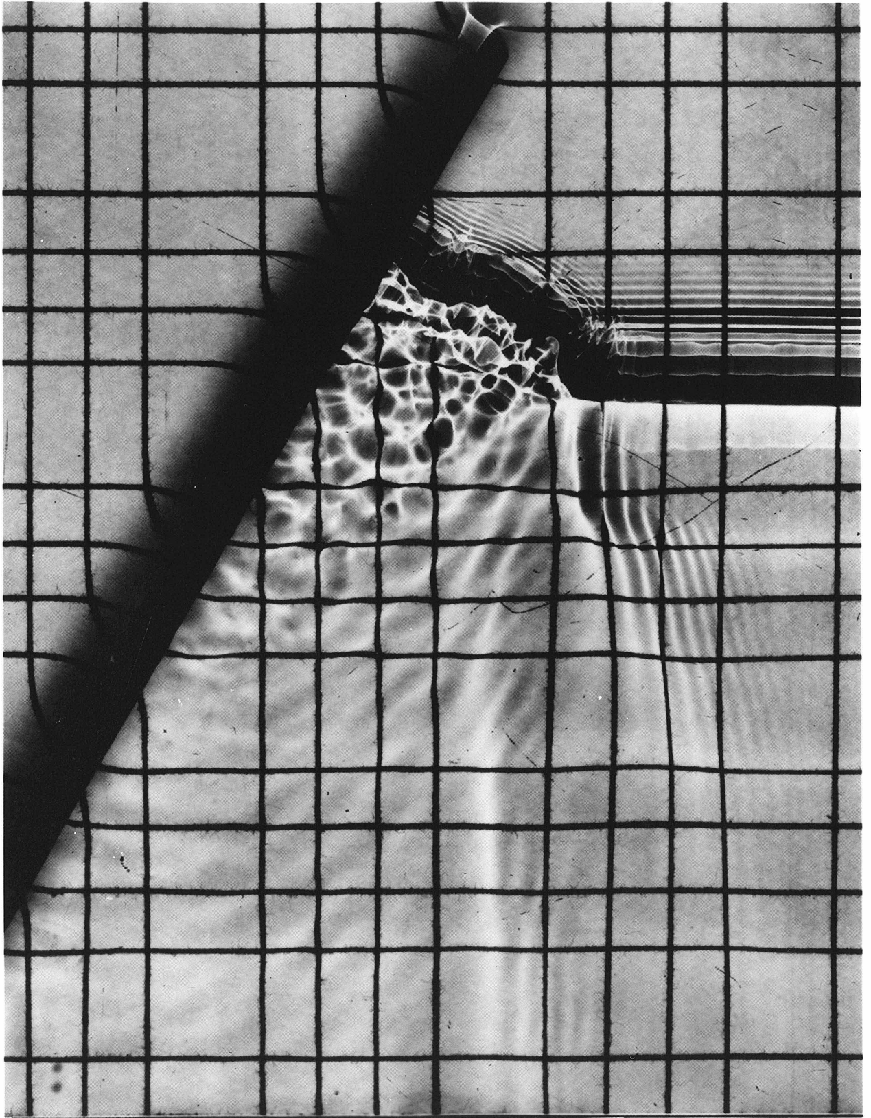
Fig. 35 Photogram of Hydraulic-Jump Reflection from Wall. \xi = 0.45 , \alpha = 61^\circ .
