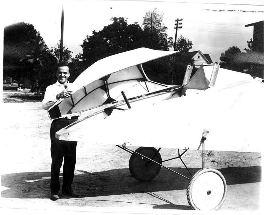
Photo 24 Showing Landing Gear - Turtleback and Fuselage under wing.
