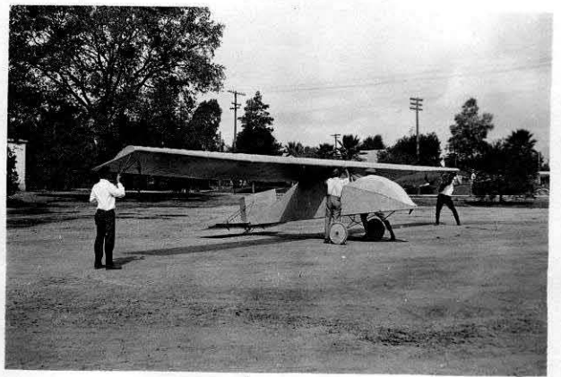
Photo. 15. Putting Wing on Fuselage.
