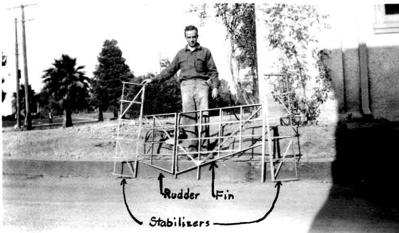
Photo 25 showing Fin, rudder & stabilizers.
