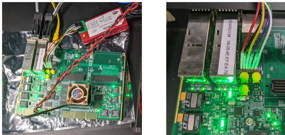
Figure A.3: Images of the JTAG device connected to a SNAP2 board.
