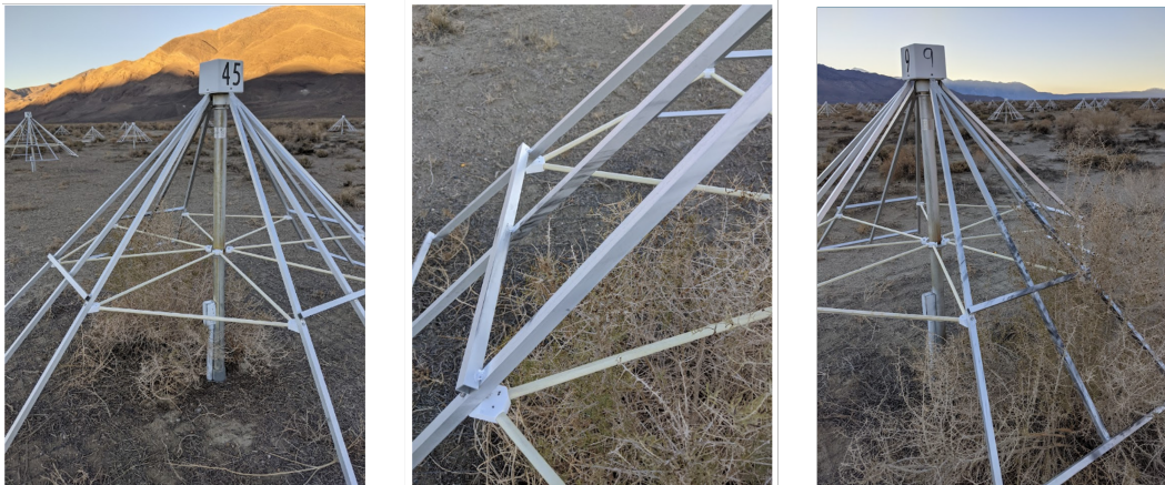
Figure 2.18: Left: Image of antenna 45 with shrub growing in it. Center: Close up photo of dipole 45A. Note the marks on the antenna. Right: Antenna 9.
