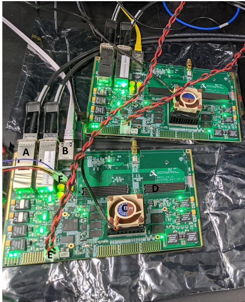
Figure 2.4: SNAP2 boards set up in the lab for testing before being installed in the OVRO-LWA. Black letters label certain important features: A) 40 Gb QSFP+ Ethernet ports. B) 1 Gb Ethernet ports. C) The Xilinx Kintex Ultrascale+ FPGA is under this heat sink and fan—the fan is used in the lab only, since in the OVRO-LWA cooled air flows through the entire electronics rack. D) One of two FPGA-mezzanine-card (FMC) connectors. Four ADC cards digitizing 16 signals each attach to each board, with a stacked pair of ADC cards attaching to each FMC connector. E) Power supply connector. F) Pin header for programming the board via JTAG. After using JTAG to load an initial firmware configuration, subsequent re-programmings can be achieved using the 1 Gb Ethernet interface.
