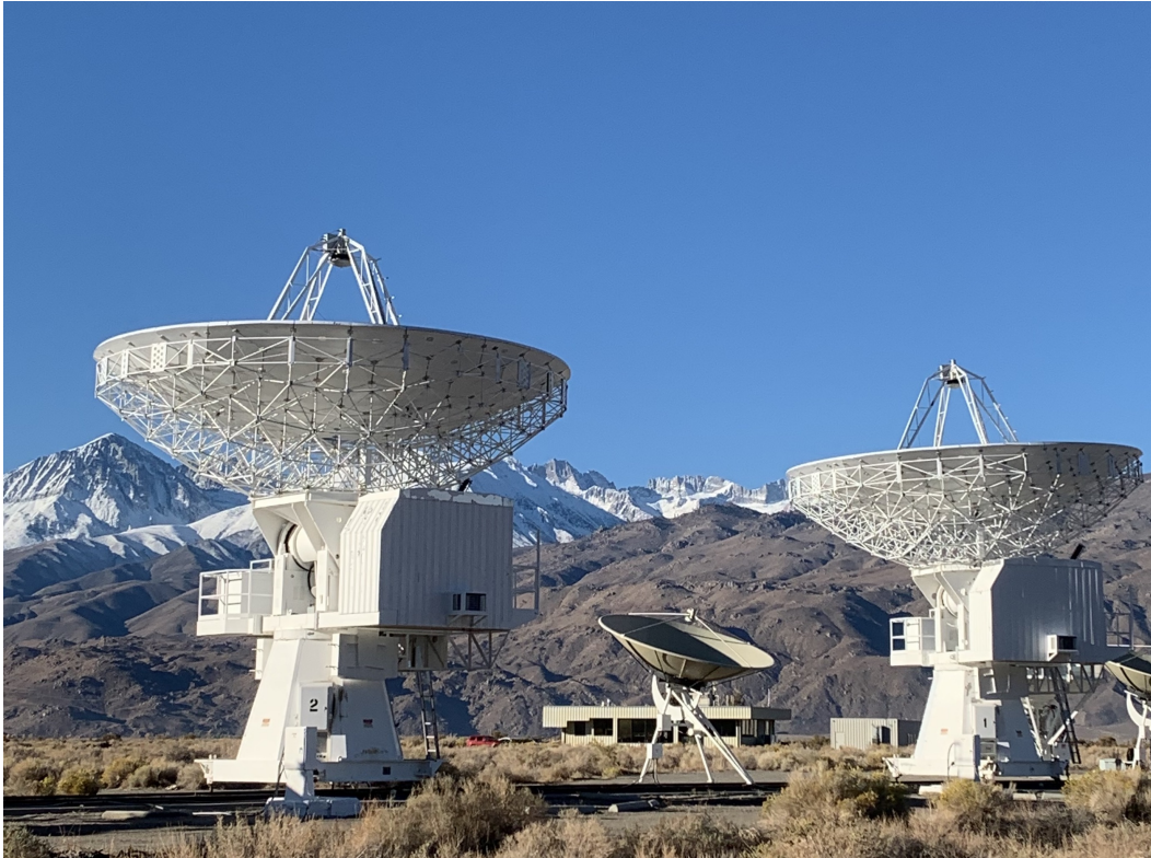
Figure 1.2: Two Leighton antennas that comprise the single baseline of SPRITE.
