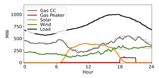
Figure 3.2: DA (dashed line) and optimal RT (solid line) dispatch trajectories for generators and load over a 24 hour scheduling horizon.
