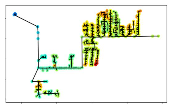
Figure 8.7: Voltage magnitudes in the PWP feeder. Blue indicates overvoltage and red indicates undervoltage. Green is approximately 1 p.u. A significant number of nodes in the feeder experience undervoltage while the substation voltages are above the nominal range.
