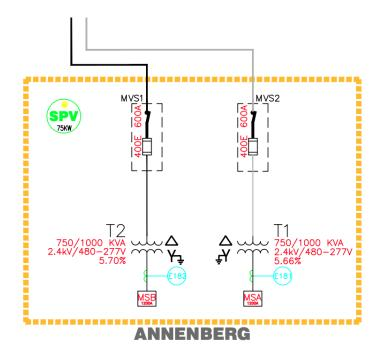
Figure 6.5: Annenberg Center single-line diagram. The solar PV (SPV) connects to MSA. The black and grey incoming feeders link the buildings to Substation 2.
