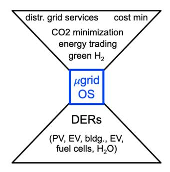
Figure 1.5: An hourglass architecture for DERs. The layered structure enables energy services to be defined without explicitly referencing the hardware that provides them. A software layer (Microgrid OS) is necessary to connect the hardware to the services.
