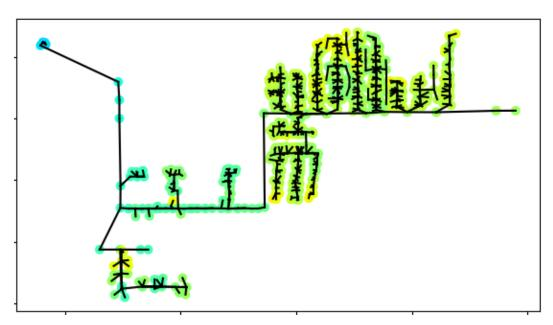
Figure 8.9: Voltage magnitudes in the PWP feeder. Blue indicates overvoltage and red indicates undervoltage. Green is approximately 1 p.u. All nodal voltages are corrected to within  $\pm 5\%$  p.u. when batteries are discharged optimally at peak feeder load.
