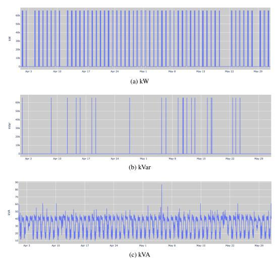
Figure 6.3: 5-min resolution kW, kVar, and kVA data from a meter in Annenberg Center, April - May 2021. Non-physical values for active and reactive power suggest sensor, communication, or database configuration errors within the BMS.
