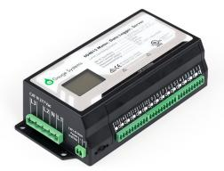
Figure 6.4: Egauge meter Model EG4015 has inputs for 15 CTs and 4 voltage connections for 480V phase-to-phase.
