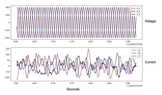
Figure 6.12: Waveform capture data for a 0.35 second window. The horizontal axis are Unix Epoch timestamps.
