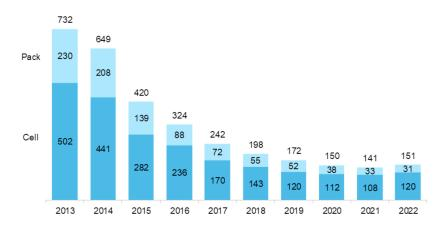
Figure 5.2: Average lithium-ion battery prices from 2013-2022 in \$/kWh [17]. Both cell and pack costs have enjoyed similar magnitude decreases in unit costs.
