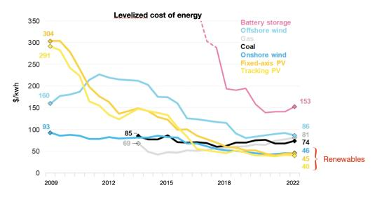
Figure 5.3: Levelized cost of energy (LCOE) in \$/kWh for various generation technologies in the US, 2009-2022 [16]. Onshore wind and utility-scale solar have the lowest LCOE of any generator types since 2018.
