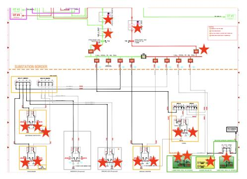
Figure 6.10: Singleline diagram of the Substation 3 sub-network with eGauge meter locations indicated by red stars.
