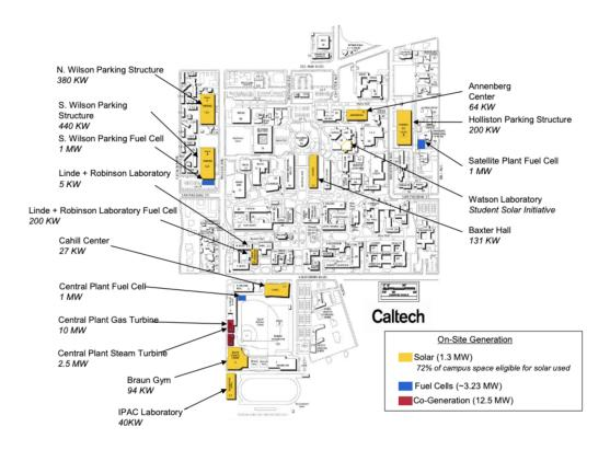
Figure 5.7: Map of Caltech Microgrid power generation assets. Source: 2020 Caltech Facilities Master Plan
