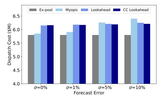
Figure 3.3: Total dispatch cost of the different pricing schemes under increasing forecast error. Forecast error is defined as the mean absolute percentage deviation from the true trajectory realization.
