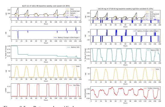
Figure 8.5: Battery charge/discharge schedules and state-of-charge trajectories optimized for time-of-use energy cost minimization.
