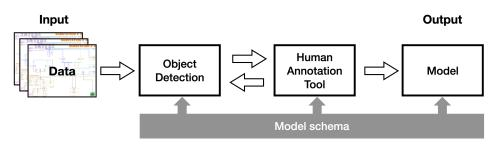
Figure 6.17: Flowchart for human-in-the-loop single-line diagram annotation pipeline.
