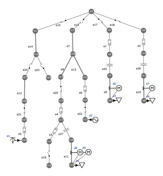
Figure 7.5: Computer-parsable singleline diagram generated from the network schema for the Kerckhoff Building at Caltech. Switch and breaker positions are taken from singleline sources but may not represent actual positions. State estimation algorithms can be used to validate or correct their statuses.
