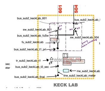
Figure 6.15: Annotated single-line diagram for Keck Lab
