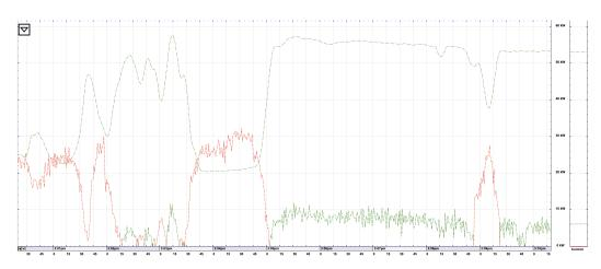
Figure 6.11: Total 3-phase power on Annenberg MSA switchboard. The upper green curve is the power generated by the rooftop PV array and red curve is the aggregate building load.
