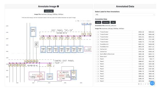
Figure 6.18: Human-in-the-loop annotation tool for single-line diagrams. The model schema is an input into the tool, limiting the available elements the annotator may select from to elements in the model.
