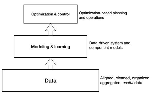
Figure 1.4: Layered architecture of the Microgrid OS. Reliable, organized, realtime data are the foundation for system models, which in turn are necessary for optimization-based control.
