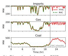
(b) Dispatch solutions for RHC vs. FFHC on a particular demand trajectory that is infeasible for RHC. Lookahead horizon is set at 1 hr for both.
