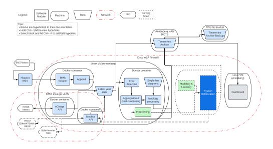
Figure 7.2: Digital Twin software system architecture block diagram.
