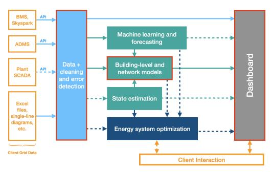
Figure 7.1: Digital Twin system architecture diagram
