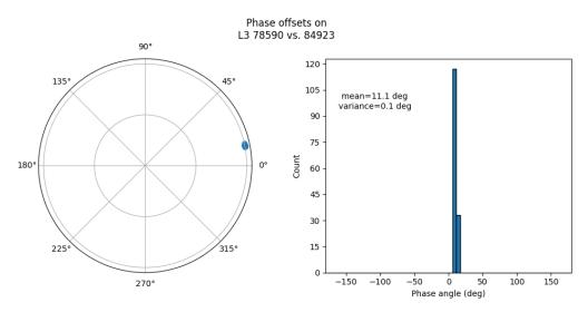
Figure 6.14: Distribution of phase offsets of the *C*-phase voltages of two meters in the Chen Neuroscience building. The meters are measuring voltages on different buses, leading to the average 11 degree phase difference between the signals. The small variance of the measurement distribution suggests accurate meter timestamp alignment.
