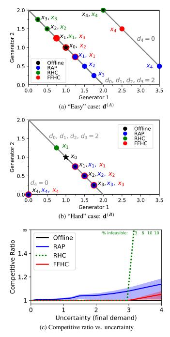
Figure 2.2: Counterexample from Theorem 1 revisited. Panel (a) shows a scenario where all algorithms are feasible. Panel (b) shows a scenario where RHC is unable to remain feasible, whereas FFHC remains feasible. Panel (c) illustrates the performance of the RHC, FFHC, and RAP against the offline optimal as the size of the uncertainty set grows. The dotted green line going to  $\infty$  indicates that RHC becomes infeasible on some trajectories beginning at an uncertainty value of 3.
