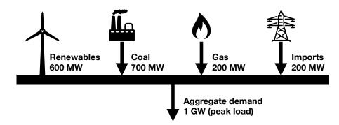
Figure 2.3: Power system for 4-generator case study. Capacities shown are peak values.
