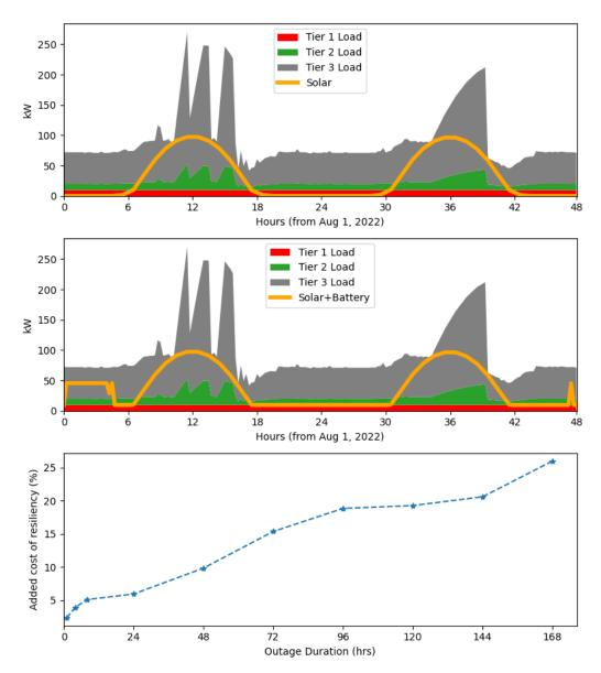
Figure 8.4: Simulation of battery and load microgrid operation at Baxter Hall over 48 hours in August 2022. The first panel shows nominal operation with significant curtailment of critical load. The second panel shows optimal discharge of the battery to meet critical and priority loads when PV generation is not available. The last panel shows the added cost of resilience that a battery incurs over the building's energy cost baseline (and over the ~15-year lifespan of the battery).
