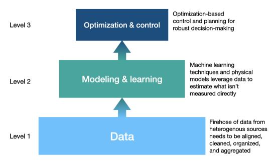
Figure 5.6: Three core functionalities of the Microgrid OS
