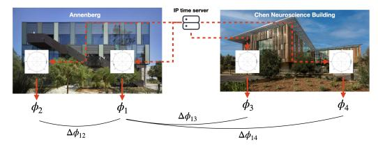
Figure 6.13: Schematic of phase offsets between meters in different locations within the electrical network, synchronized via network time servers.
