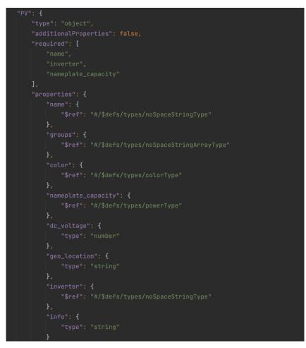
Figure 6.16: json schema object for a PV array.
