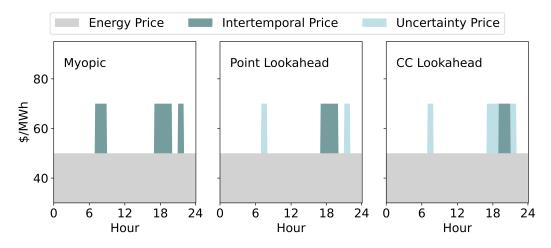
Figure 3.4: Price trajectory  $\pi_{i,t}^*$  for the gas combined-cycle generator under  $\sigma = 10\%$  forecast uncertainty for different real-time forecast methodologies.
