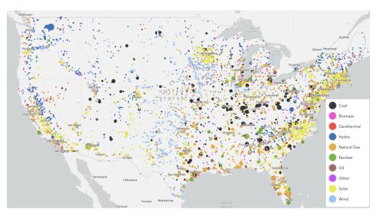
Figure 1.2: Map of generating plants in the US in 2023. Solar and wind are in yellow and blue circles, the size of which represents the size of the power plant [126]. The typical gas or coal power plant is between 500-1000MW, whereas the average size of a solar generator is 1-5MW.
