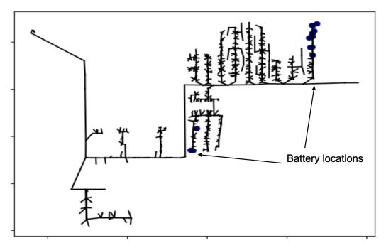
Figure 8.8: Dark blue circles show the optimal battery placement locations. The selected nodes are typically at the end of long or over-loaded lateral lines in the feeder.
