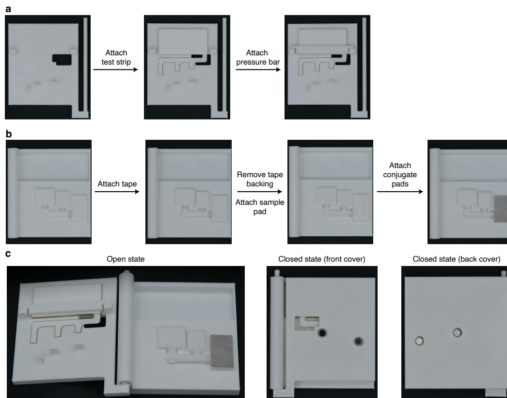
Figure C.6: Steps for assembling the folding card device for viral protein detection. (a) Assembling the left page. The adherent backing on the nitrocellulose membrane and wicking pad is removed, and the bottoms of the three nitrocellulose membrane channels are aligned with the thin markers on the device before adhering the nitrocellulose membrane and wicking pad in place. The pressure bar is added by pushing its two cylindrical prongs into the holes on either side of the wicking pad. (b) Assembling the right page. Double-sided tape is applied to the sample pad and conjugate pad pedestals. The adherent backing is removed from the double sided tape, and the sample pad is affixed to the sample pad pedestal. The conjugate pads are then applied to the conjugate pad pedestals, with their leading edges overlapping with the sample pad by 2 mm. (c) The left and right pages of the folding card device are assembled at the hinge. Images depict the device in the open state (left) and in the closed state viewing either the front cover (middle) or back cover (right).
