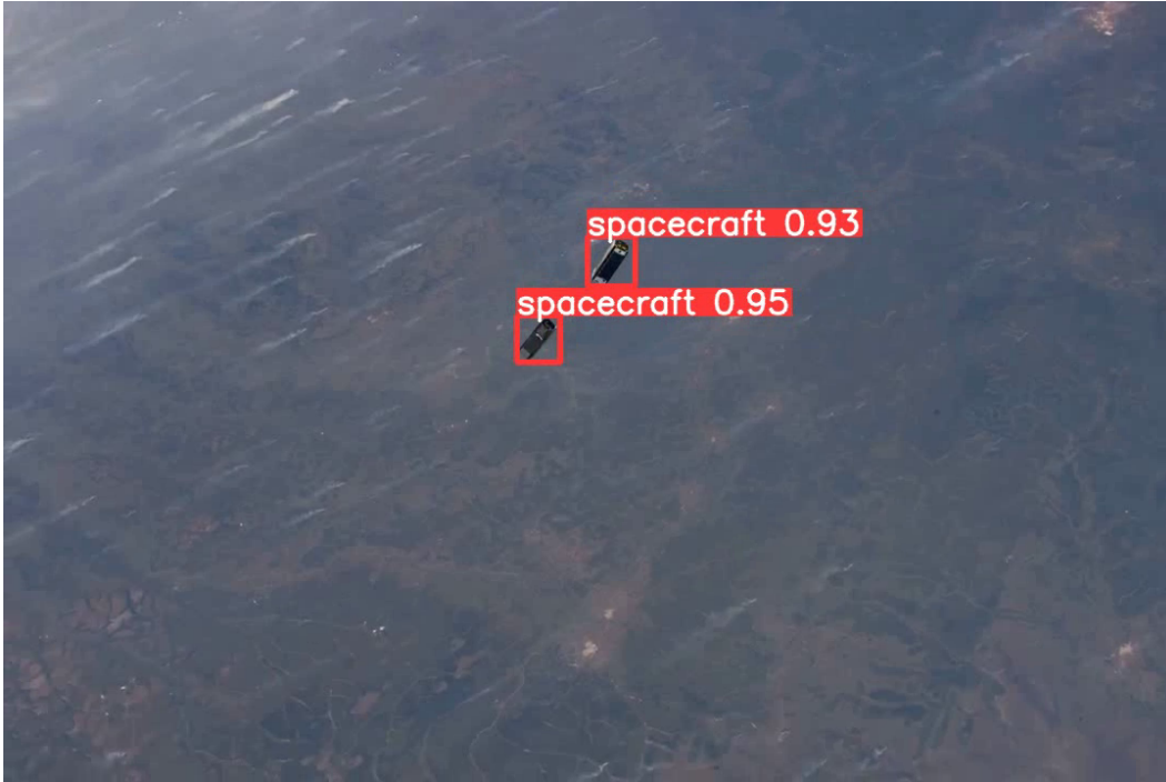
Figure 5.13: Spacecraft detection algorithm classifying MinXSS (bottom) and CADRE spacecraft (top) from the real images taken from the International Space Station.
