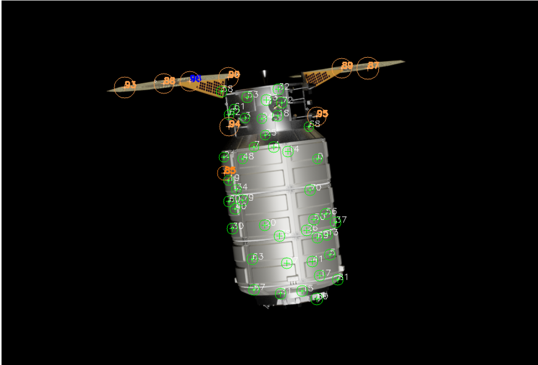
Figure 4.6: Tracked landmark overlaid on the synthetic image. Circles around each landmark indicate the size of uncertainties. Green landmarks indicate states that are tracked for more than 10 consecutive frames.
