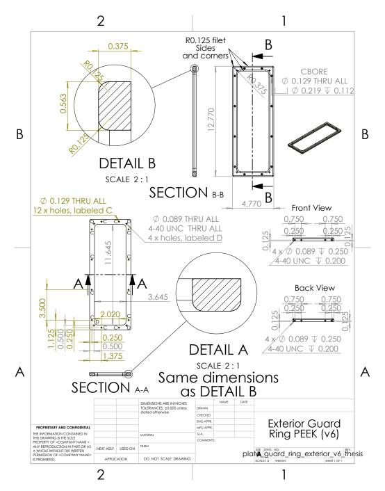
Figure F.3: Design of the exterior PEEK guard ring holding the E-field plates. See main text for details.
