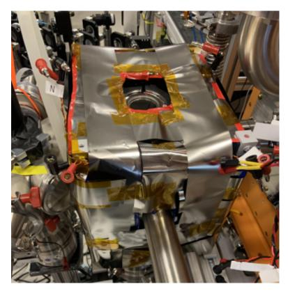
Figure 5.6: A photo of the home-made magnetic shielding around the six-way KF50 cross. See main text for details.
