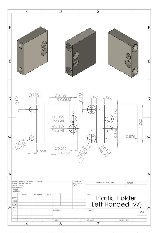
Figure F.5: Design of the left-handed PEEK holder connecting the exterior guard ring to the support and spacer rods. See main text for details.
