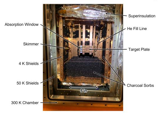
Figure 3.2: A photo of the 4 K CBGB source with labeled components. This photo was taken after the cryo-pumping upgrades described in the section on cryopumping. The cell sits in the middle of the photo, anchored with vertical bars to the top of the 4 K shields, which is connected to the cold head (not visible). See main text for more details.
