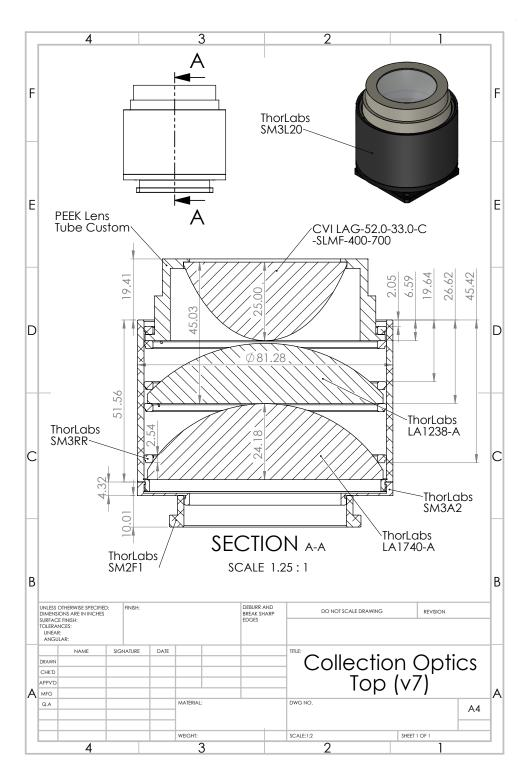
Figure F.9: Design of the top collection optics stack. Light pipe not shown. Il lens tubes are not black anodized. See main text for details.
