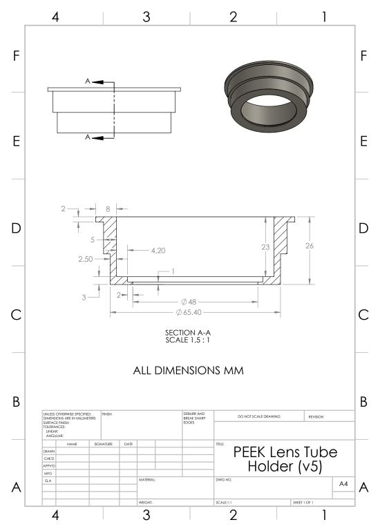
Figure F.11: Design of the PEEK lens tube holder for the collection optics stacks. See main text for details.
