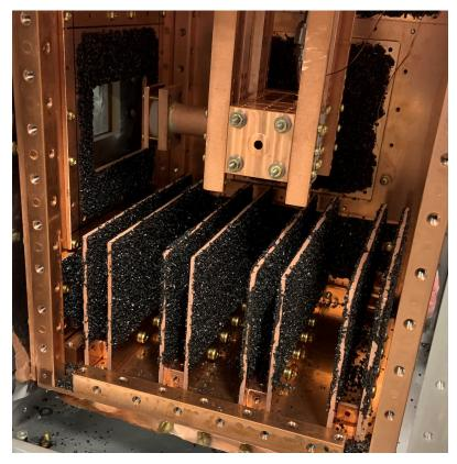
Figure 3.4: A photo of the charcoal sorb fins after installation. The fins are mounted to the bottom of the 4 K radiation shields. The cell is visible, along with the exit aperture and the ablation snorkel, which is used to prevent the ablation plume from coating the ablation window. Charcoal sorbs on the sides of the 4 K chamber are also visible.
