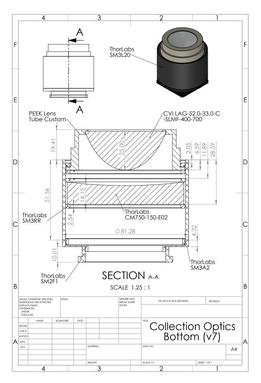
Figure F.10: Design of the bottom retro-reflecting optics stack. See main text for details.
