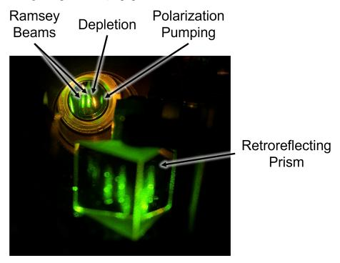
Figure 5.22: A photo of the laser beams used to perform Ramsey interferometry. The beams are cylindrically shaped to cover the entire molecular beam. The molecules first encounter polarization pumping, followed by depletion, and then Ramsey beams. See main text for details. Readout is not pictured. The retroreflecting prism used to generate the second Ramsey beam is visible.
