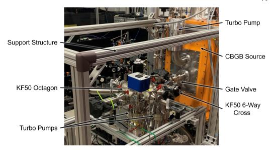
Figure 3.3: The beam extension downstream from the CBGB source. This photo was taken with many electronics, optics, and detectors removed.
