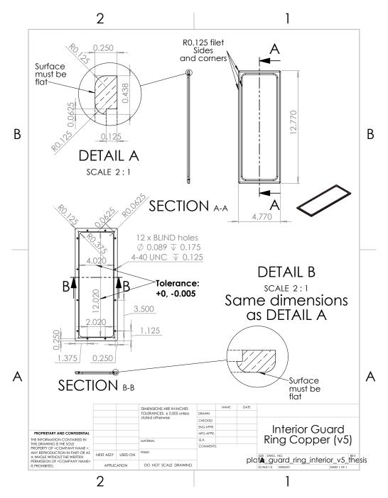
Figure F.4: Design of the interior copper guard ring holding the E-field plates. See main text for details.
