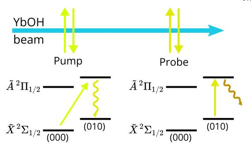
Figure 4.15: Schematic of the beamline used for tests of optical pumping into the  $\tilde{X}(010)$  state and characterization of  $\tilde{X}(010) \to \tilde{A}(010)$  lines. Upstream, the molecules are pumped out of  $\tilde{X}(000)$  through the excited  $\tilde{A}(010)$  state, decaying into  $\tilde{X}(010)$ . Downstream, we probe the increased fluorescence in the  $\tilde{X}(010)$  state using the diagonal transition to  $\tilde{A}(010)$ .
