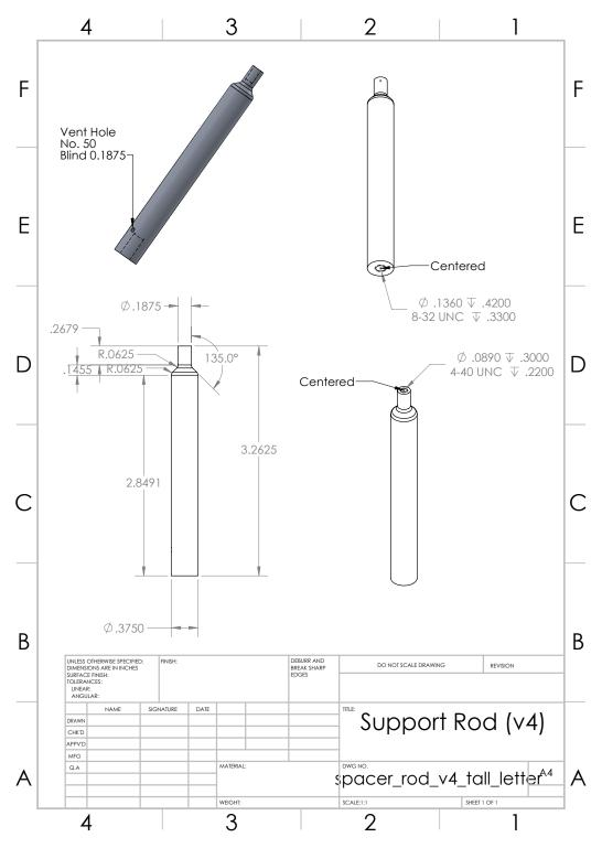
Figure F.7: Design of the support rods holding up the E-field plates. See main text for details.
