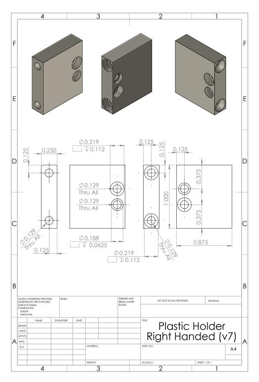
Figure F.6: Design of the right-handed PEEK holder connecting the exterior guard ring to the support and spacer rods. See main text for details.
