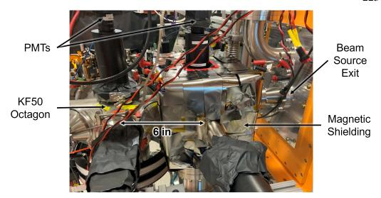
Figure 5.13: A photo of the beamline used for the two-photon tests. The molecule beam exits the beam source on the right and travels toward the left. The region wrapped in magnetic shielding contains the upstream KF50 cross and the 3-axis square magnetic field coils, and is where the two-photon tests occur. The downstream octagon is where we perform state readout and collect LIF. The 6 inch scale indicated is approximate.
