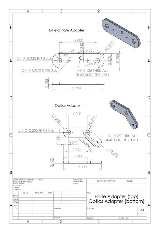
Figure F.12: Design of the aluminum adapter plates connecting the support rods to the IdealVac chamber hole pattern (top, E-field plate adapter), and connecting the optics stacks to the IdealVac chamber hole pattern (bottom, optics adapter). See main text for details.
