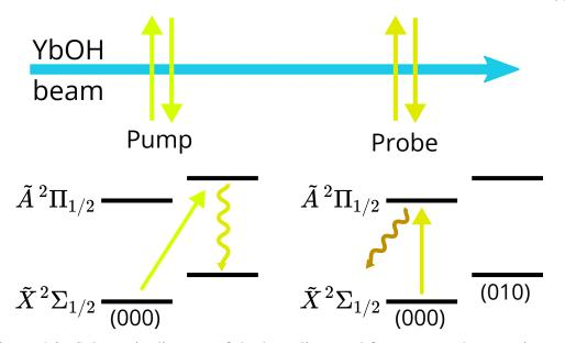
Figure 4.9: Schematic diagram of the beamline used for pump probe experiments to study the  $\tilde{X}(000) \to \tilde{A}(010)$  transition. Upstream, the pump light is scanned. Downstream, the probe light monitors a single rotational level in  $\tilde{X}(000)$ . If the pump laser hits a resonance, we will see fluorescence in the pump region. Furthermore, if the pump addresses the same ground state as the probe, then we will observe correlated loss of the probe fluorescence.
