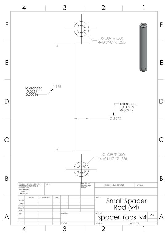
Figure F.8: Design of the spacer rods that separate the two E-field plates. See main text for details.
