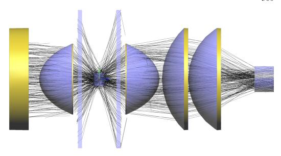
Figure F.2: Simulations of the fluorescence collection setup for the science chamber. Simulations were performed using LightTools. The diagram here only shows transmitted and totally-internally reflected rays. See main text for details.
