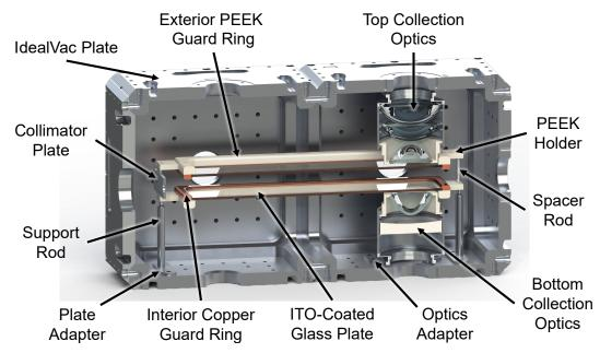
Figure F.1: Annotated render of a cut-away view of the MQM science chamber. The molecule beam travels from left to right. Unless stated otherwise, all parts are aluminum 6061 construction. The bottom collection optics retroreflects the fluorescence light. The top collection optics focuses the light into a light pipe, not pictured.
