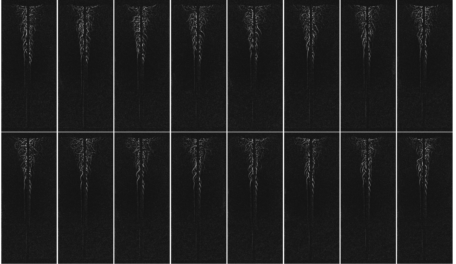
Figure 6.8: Processed Shadowgraph image sequence from T_w = 555 K for H28 cylinder. Fluctuations and transition is mostly located in the upper region of the surface. Early vortex formation is seen occurring over the course of many frames on the right side of the cylinder near the middle of the frame. \Delta t between frames is 1/30 s. Note: Images have been brightened and contrast stretched for presentation.
