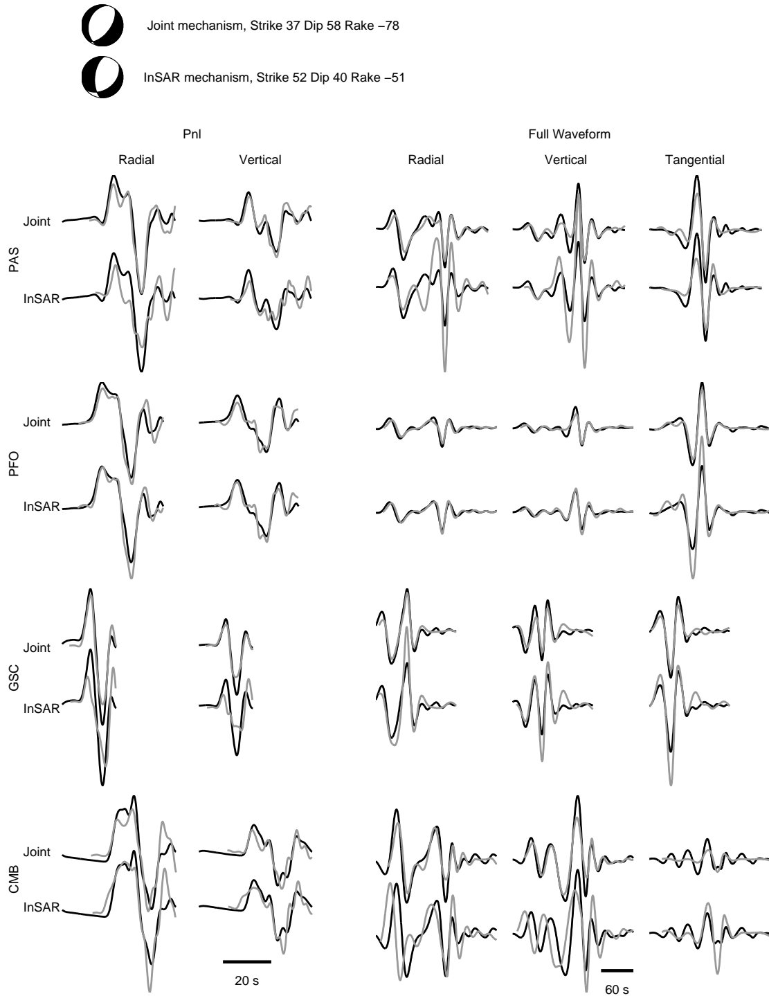
Figure 2.5: Mechanisms, observed waveforms, and synthetic waveforms from the joint and InSAR-only inversions using the Mojave layered model. Pnl waveforms are filtered from 0.01-0.2 Hz, while full waveforms are filtered from 0.01-0.05 Hz. Data are shown as black lines and synthetics as gray lines. The time scale is shown at the base of each group of plots, with the 20 second bar referring to the Pnl waveforms and the 60 second bar referring to the full waveforms.
