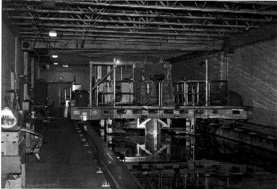
(a) Front view of towing carriage at one end of the tank. The wedge model can be seen suspended from the carriage hanging into the water at the center of the tank.
