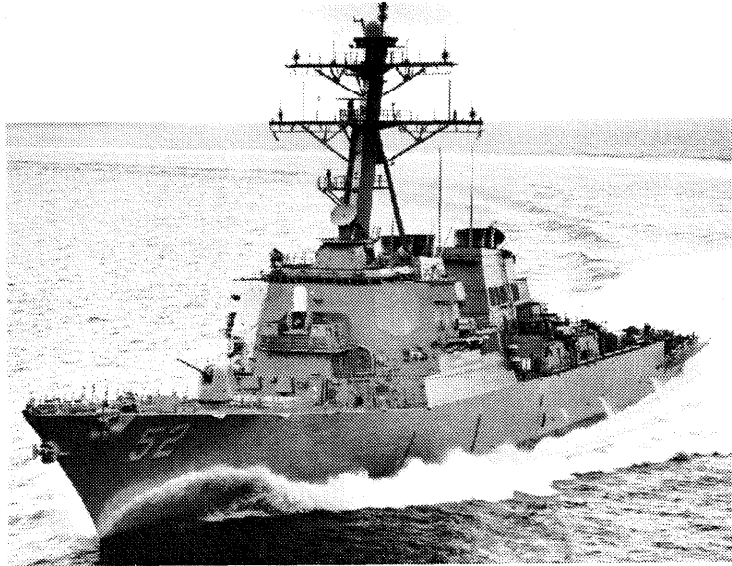
(a) USS Barry (DDG52), christened 4/23/94. The hull length is 506 ft., and the navigational draft is 32 ft.
