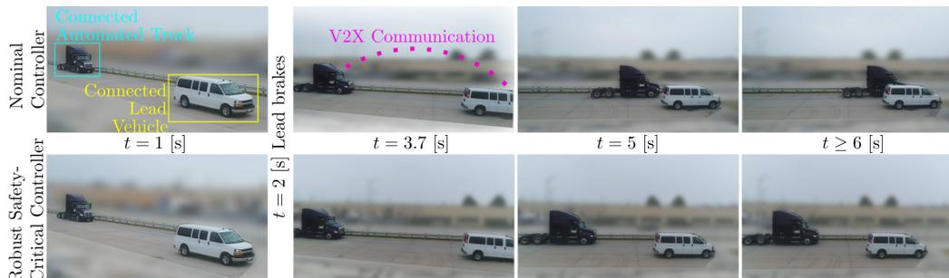
**Figure 4.8.** Experimental configuration for heavy-duty semi-trailer truck problem. (Top) Controller design without robustifying element yields safety violation. (Bottom) Robust safety-critical controller ensures semi-trailer truck brakes early and aggressively enough to maintain safe distance.
