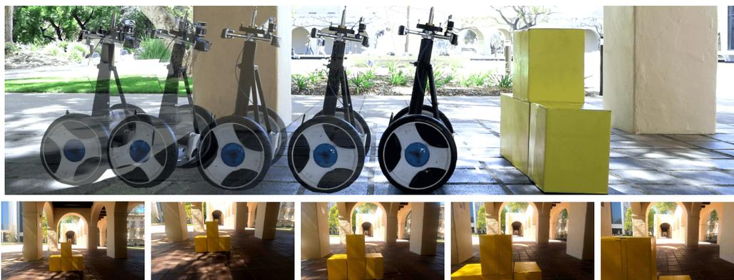
**Figure 5.5.** Images from the experiment using the (MR-BS-SOCP) controller. The Segway is piloted towards a wall of yellow boxes and the controller ensures that it remains safe, i.e. that it does not crash into the boxes. (Top) Time lapse of the Segway trajectory. (Bottom) Camera images taken from the perspective of the Segway throughout the experiment. The images are displayed in chronological order from left to right. A video can be found at <https://vimeo.com/520247516>.
