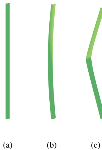
Figure 4.10: Tape spring with parameters L = 300 mm, R = 10 mm and t = 0.1 mm. (a) Initial state. (b) Deformed state before snap-through. (c) Final deformed state.
