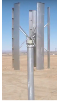
Figure 4.2: Photographs (left) and specifications (right) of the helical-bladed UGE turbine (top) and the straight-bladed WPE turbine (bottom). The blade twist of the UGE turbine is \tau = 0.694 \text{ rad} \cdot \text{m}^{-1} .
