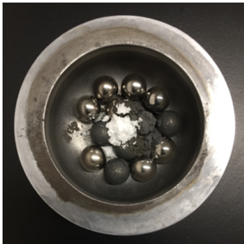
Figure 3.5: Ball milling vial prior to milling, with steel balls, sample powders, and stearic acid (white powder).
