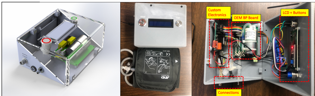
Figure A.4: Second device build and measurement. (Left) shows a 3D rendering of the CAD model from isometric view with transparent top cover. (Middle) shows the device enclosure from a top view with the cuff. (Right) the electronics of the device safely placed within the enclosure.
