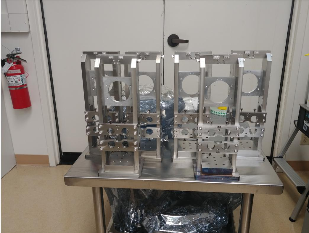
Figure A.2: SOS towers prepared for suspending optics.
