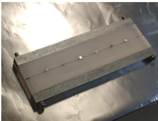
Figure A.1: Gluing dumbbells to magnets for suspensions. The North and South poles of the magnets are segregated and placed on the fixture. Dumbbells with small amount of EP-30 glue is placed on the top and left to cure for 24 hours.
