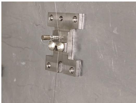
Figure A.3: Side plate for attaching wires and side magnet for 2" to 3" adaptor.
