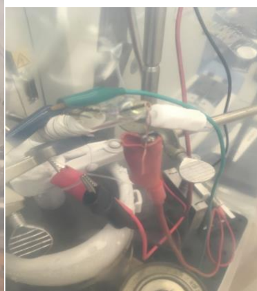
Figure 2.1: Exterior of plastic shroud covering DART inlet. Figure 2.2: DART inlet beneath shroud. Figure 2.3: Close-up of DART ionization source.
