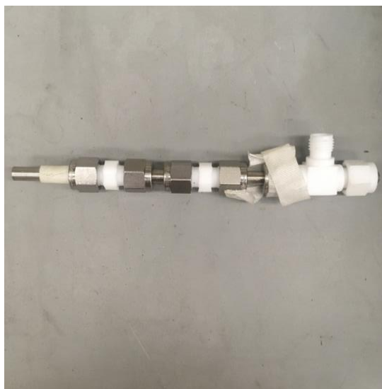
Figure 2.5: Photograph of stainless steel DART inlet.
