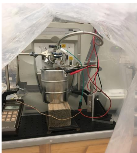
Figure 2.1: Exterior of plastic shroud covering DART inlet. Figure 2.2: DART inlet beneath shroud. Figure 2.3: Close-up of DART ionization source.
