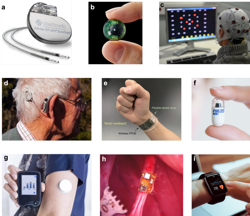
Fig. 1.1: Medical electronic devices for a variety of applications: (a) pacemaker, (b) eye implant for smart vision, (c) brain-machine interfaces, (d) cochlear implants, (e) smart electronic wristband, (f) PillCam for capsule endoscopy, (g) continuous blood glucose monitoring patch, (h) neural stimulator IC, and (i) smart watch for health monitoring.
